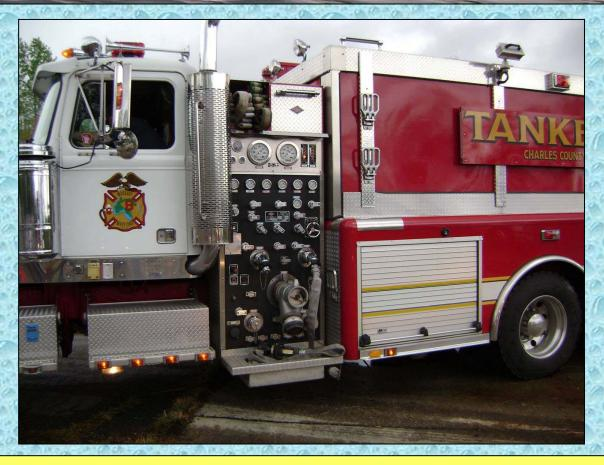
Although a water hauling rig primarily, Tanker 8 has a 750 gpm pump and a couple of pre-connected attack lines if fire attack operations are needed.
