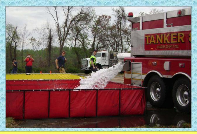
Tanker 8 is shown here at a water supply drill in Prince George's County off-loading water through a side dump.
