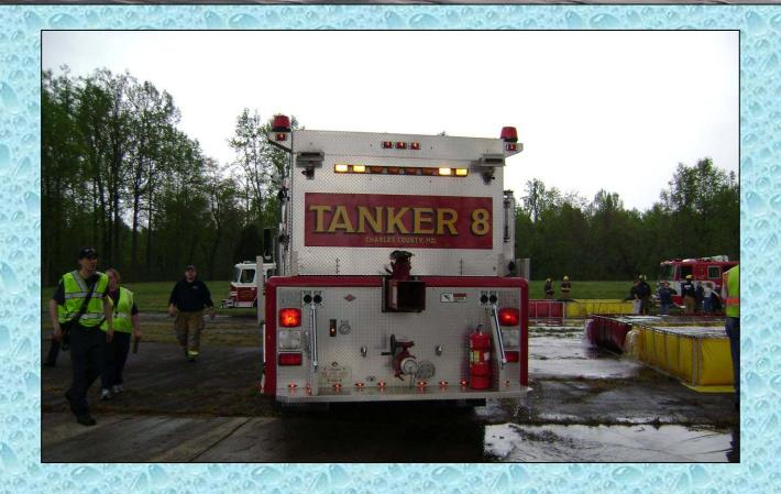
The tanker has both side and rear dumps and a large, direct fill line controlled with a butterfly valve.
