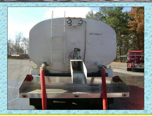
The tanker was retrofitted with a big dump valve and direct fill lines so that it could serve as a FD tanker.
