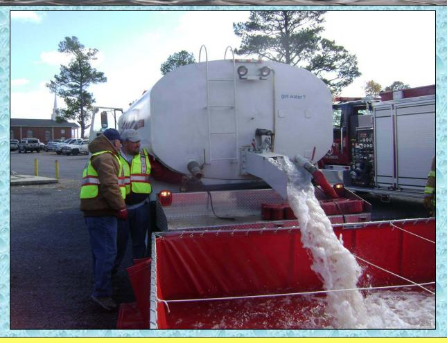
The tanker's 10-inch dump off-loads the rig's 3,750-gallons in a very short time.
