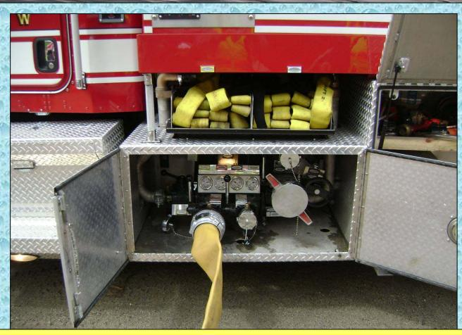
40-W-1 (Tanker 1) is outfitted with a PTO-driven, 500 gpm pump that is packaged in a space-efficient manner.
