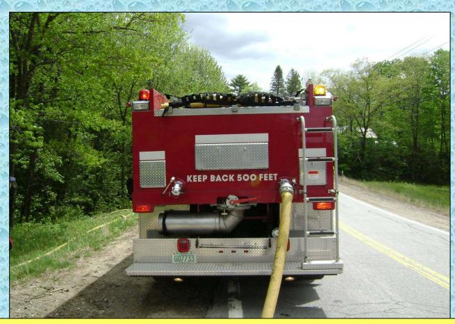
The tanker has a 2-1/2-inch and a 4-inch direct fill line. The 4-inch line is shown in use above at a water supply drill.
