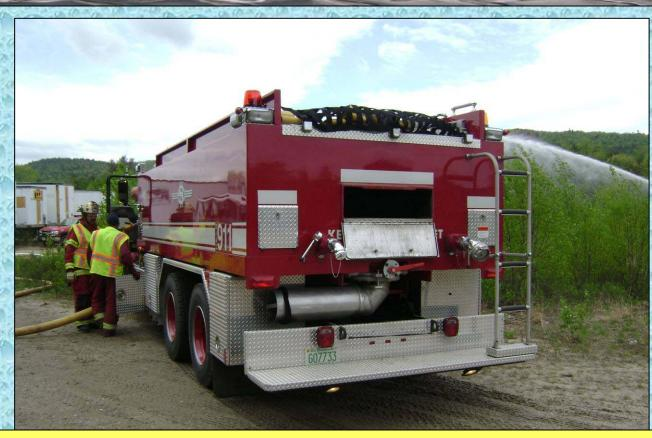
Another unique feature of this tanker is the pivoting dump valve/chute on the rear of the rig. The 12-inch dump can be pivoted to various positions as needed - which improves the versatility of the tanker. The tanker also carries a 3,500 gallon portable dump tank (in the compartment that is open above).
