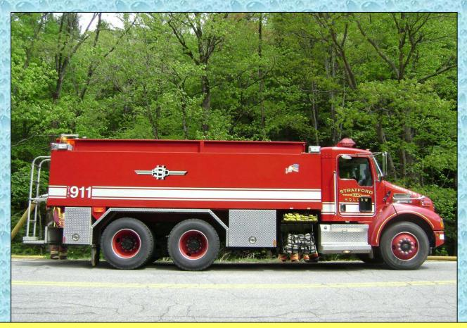
The tanker also carries some hose in a small compartment area just to the rear of the cab – an efficient use of space.
