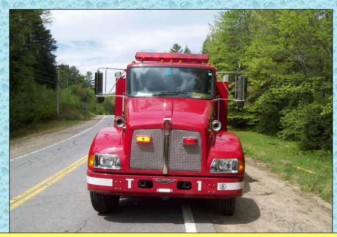
This 2007, Pierce tanker is built on a Kenworth chassis and carries 3,000 gallons of water. It is set-up to haul water and offload it quickly.
