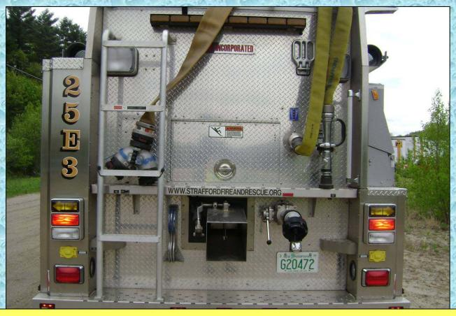
The engine/tanker has a 12-inch rear dump and a 3-inch direct fill line. The rig also carries 1,200 feet of 4-inch hose trimmed out with a double-clappered siamese to support a "rural hitch" operation.
