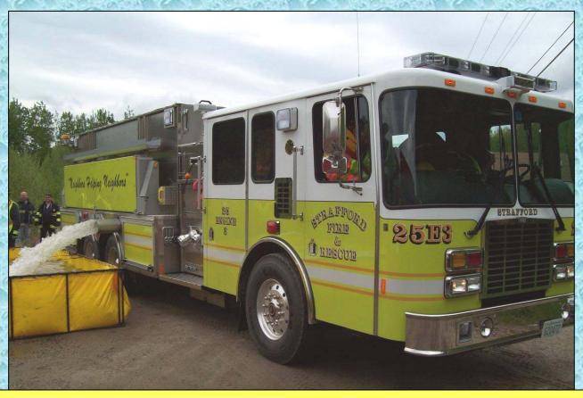
25-Engine-3 is shown above offloading its water at a water supply drill in nearby Ashland, NH. Side dumps add versatility to tankers and reduce the need to back-up or maneuver for a rear dump operation.
