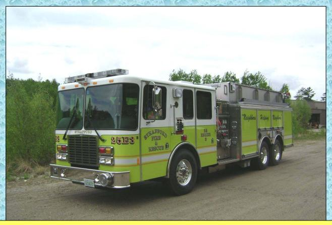
This 2007, engine/tanker is really set-up to move some "big water". Its 1,750 gpm pump combined with its 3,000 gallon water tank provide for a versatile water supply operation.
