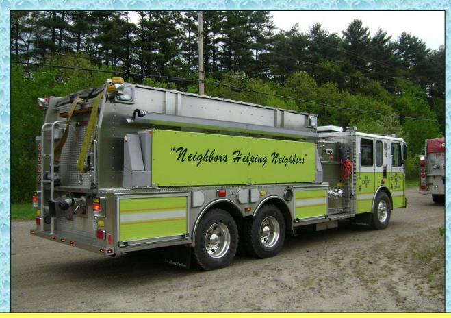
The rig carries a 3,500 gallon portable dump and is outfitted with a 10-inch dump on each side.
