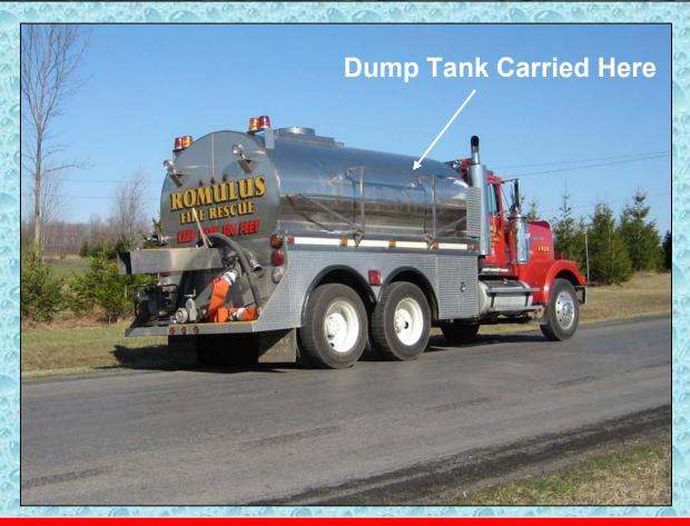
This photo was taking during a drill – so the 2,500-gallon dump tank normally carried on the side of the tanker is being used at the dump site.
