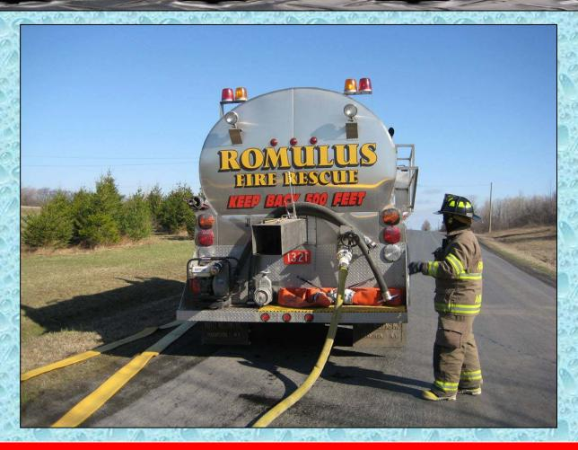
The larger direct fill lines allow for a faster fill time. FYI – the 3-inch fill hose shown in this photo was changed out for a 4-inch line later in the drill.
