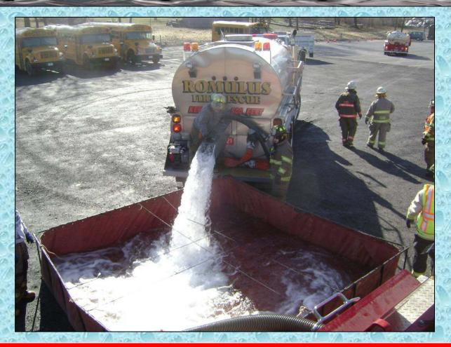
The tanker's 10-inch rear dump makes quick work of off-loading the rig's 3,000 gallons of water.
