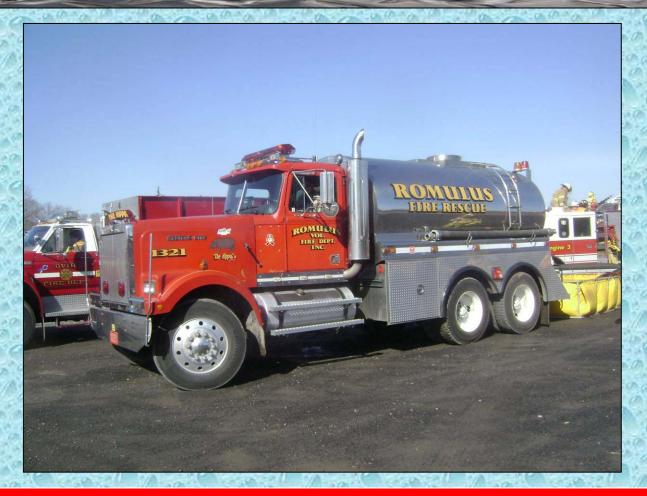
Tanker 1321's short wheel-base allows for easy maneuvering on winding and narrow roads.
