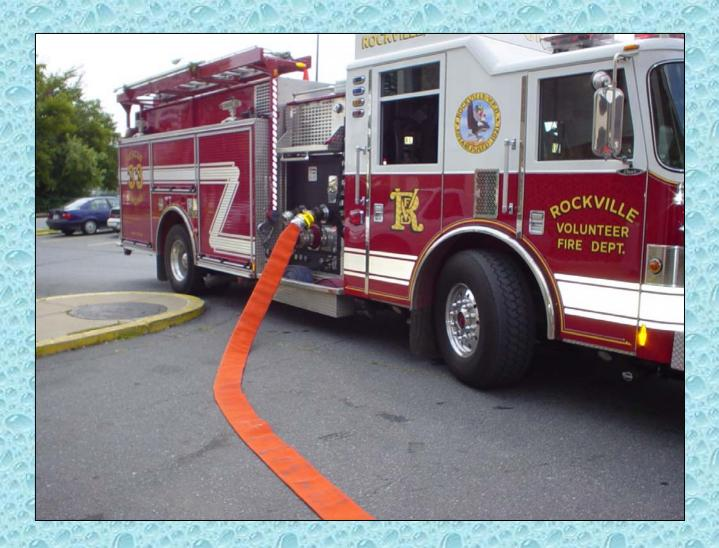
The other end of the layout feed Rescue Engine 703, a 2000 gpm pumper.
