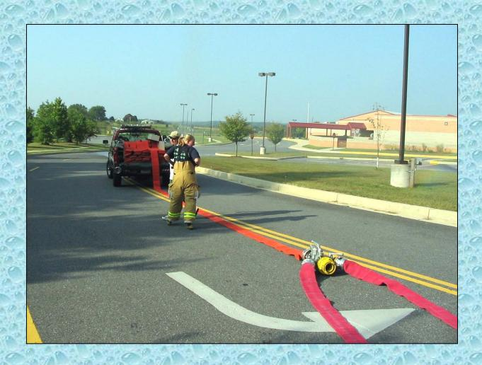
HT703 shown in action here at the 2005 South Carroll Water Supply Shuttle were it helped deploy 5-inch LDH for supplying the simulated fire attack.
