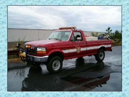
1995 Ford F250 pickup truck converted to a mini-water supply support rig
