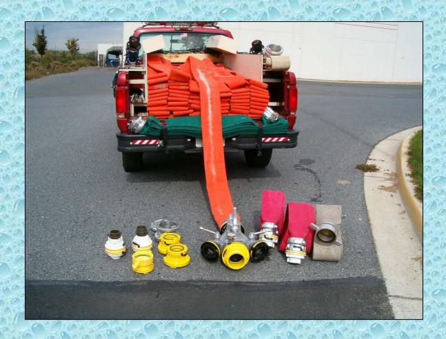
Numerous "toys" are carried in order to maximize the rig's ability to deploy and above ground, 5-inch water main.
