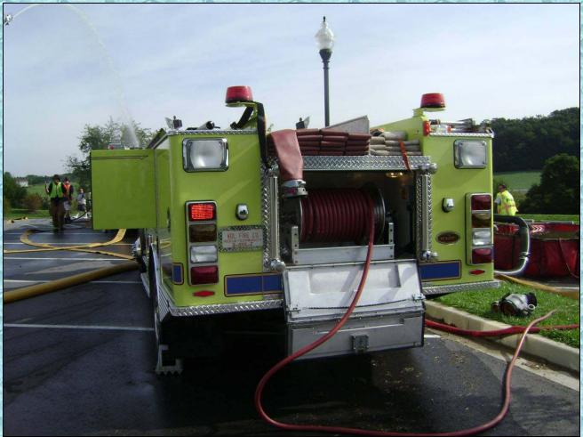
Brush 95 is shown above running jet siphons at a water supply drill in nearby Pleasant Valley, MD. The unit established a draft from one dump tank and then supported jet siphons so that water could be transferred to adjacent tanks – thus freeing up pumping capacity for the primary drafting pumper.
