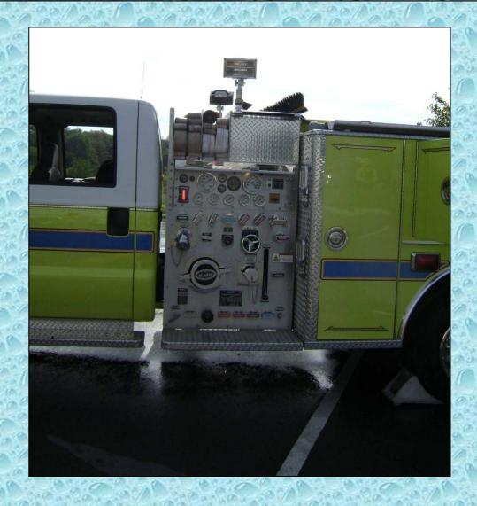
The rig was built by KME and is equipped with a Hale 1,000 gpm midship pump which can support a tanker fill site operation.
