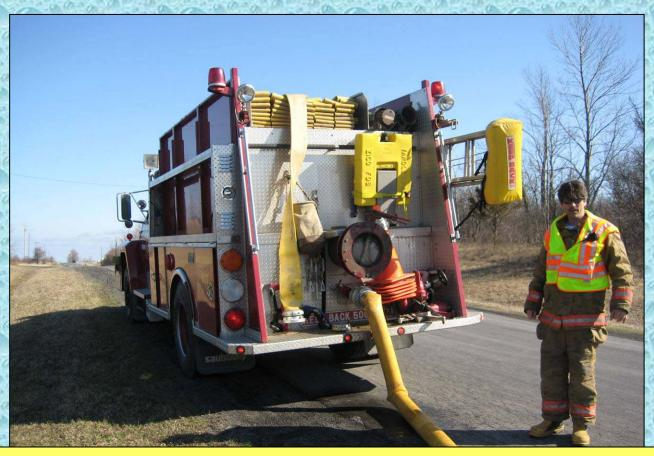
The rig is equipped with a 12-inch rear dump that offloads water amazingly fast. The pumper also has a 2-1/2-inch direct fill line outfitted with a 4-inch Storz adaptor. The pumper carries 5-inch LDH supply hose.
