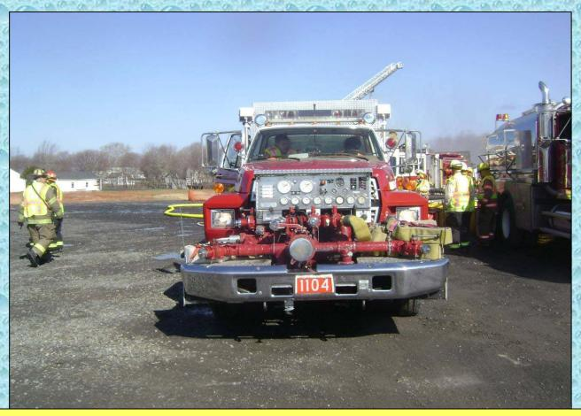
A front-mounted pump is often useful in the rural setting when access to drafting sites can be limited.
