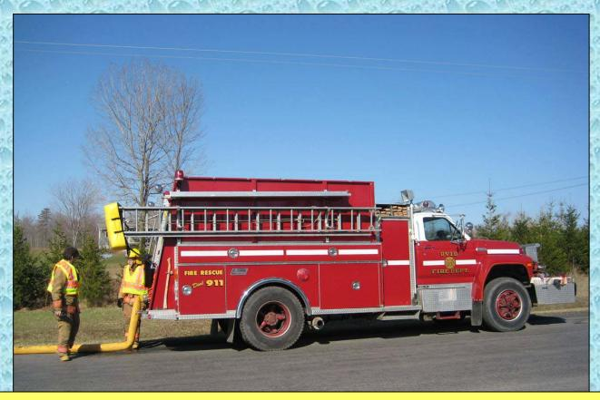
The pumper's short wheel base allows for easier maneuvering on the rural roads around Ovid. A front-mount pump allows for a shorter wheel base – but does create a bigger front "overhang."
