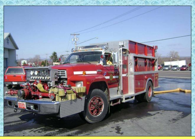
Engine 1104's pump is a 1,000 gpm pump that has been de-rated over time due to age and performance. However, it is still quite a capable unit!
