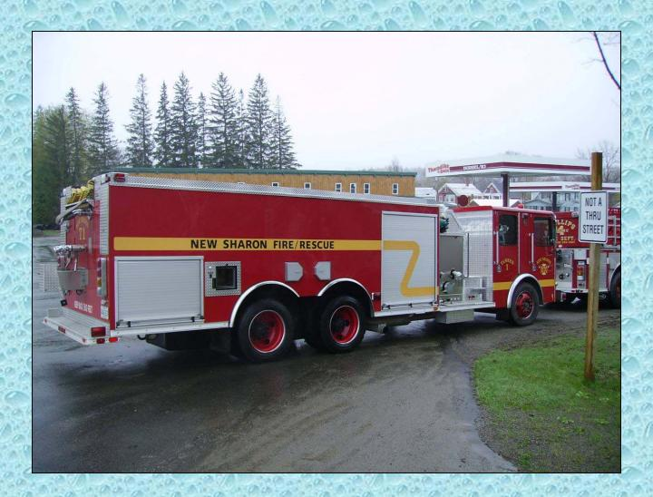
Tanker 1 has a 2,500-gallon poly tank and carries a 3,000-gallon dump tank. The tanker can dump off of both sides or the rear – all three sides are outfitted with a 10-inch dump valve/chute.
