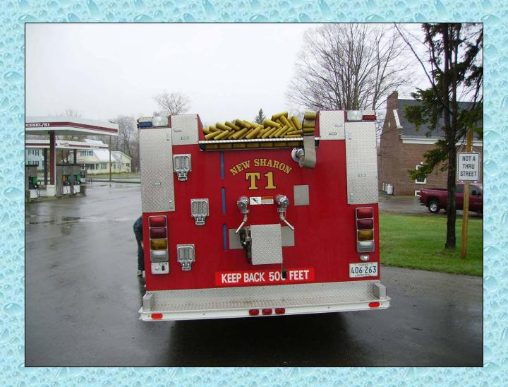
The tanker also carries 4-inch LDH supply hose as well as other basic fire fighting equipment needed to perform attack engine operations.
