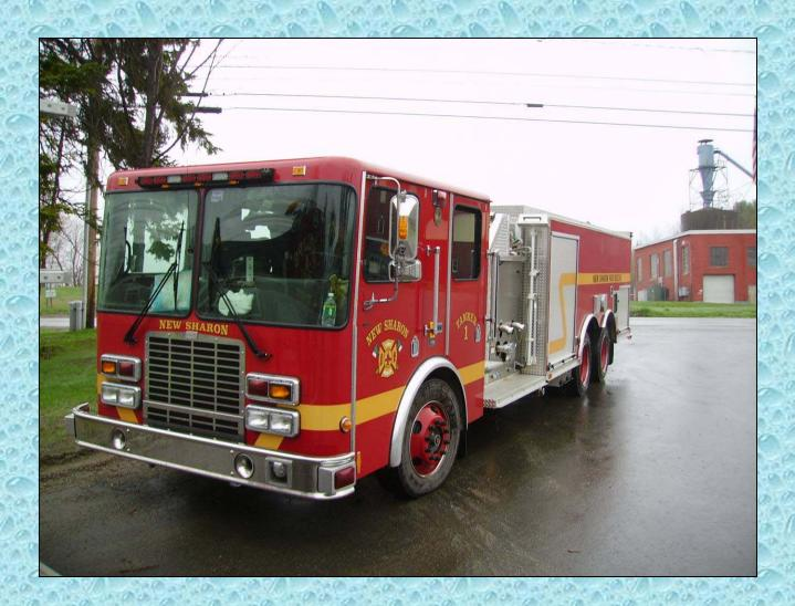
Tanker 1's low profile is designed specifically for the limited bay door height in the New Sharon fire station.
