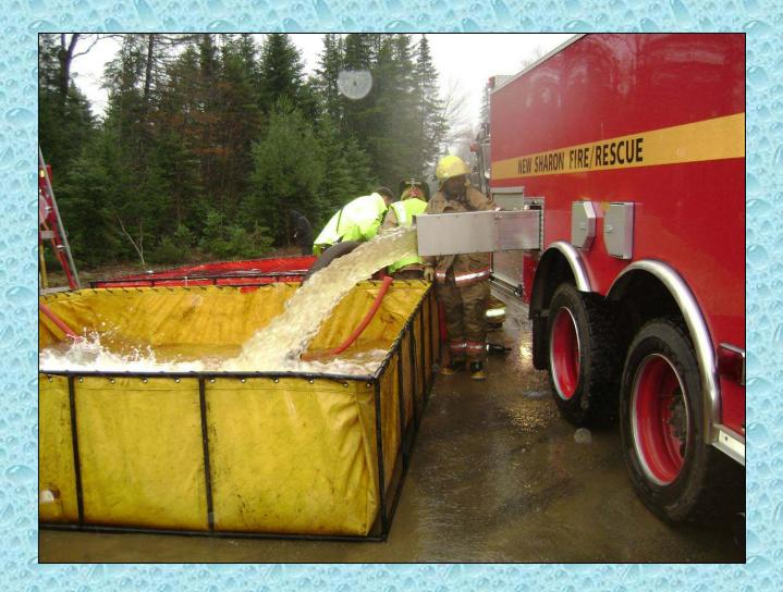
Tanker 1 is shown here off-loading water at a water supply drill in nearby Strong, Maine. The extended chute on the 10-inch dump makes off-loading much easier —especially at night..
