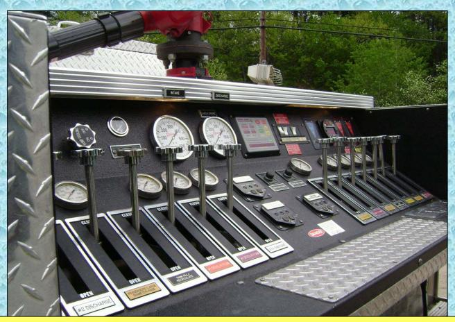
Some departments like a top mounted pump panel because it can give the operator a better view of the emergency scene.
