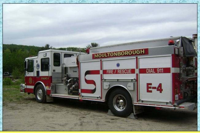
The pumper carries a full complement of engine company tools and has a 1,000 gallon water tank. The pumper also is equipped with a Class A foam system.
