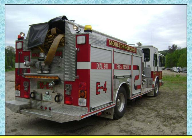
The pumper carries all of its ladders and suction hose inside compartments.
