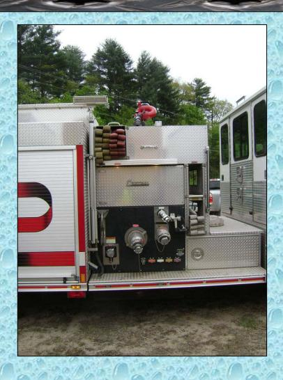
Both sides of the pump on this rig are set up to operate with large diameter hose
