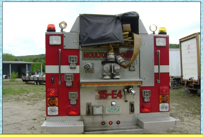
15-Engine-4 carries 1,200 feet of 4-inch hose trimmed out with a double-clappered siamese to support a "rural hitch operation". The rig also has a 2-1/2-inch direct fill line.
