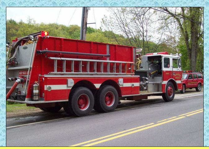
14-Tanker-5 carries 2,500 gallons of water and 1,100 feet of 4-inch supply hose.
