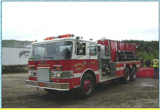
This 1988 engine/tanker is set-up to function as both an attack engine and as a water supply piece if needed.
