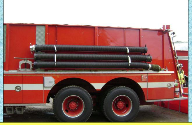
The rig also carries more than the traditional 20-feet of suction hose because folks in the rural environment know that additional suction is often needed to access draft sites or to support dump tank operations.
