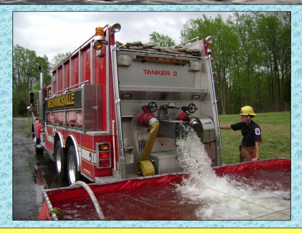
Tanker 2 is shown here off-loading water at drill in nearby Prince George's County. The tanker also has large capacity direct fill lines for quick fill operations.
