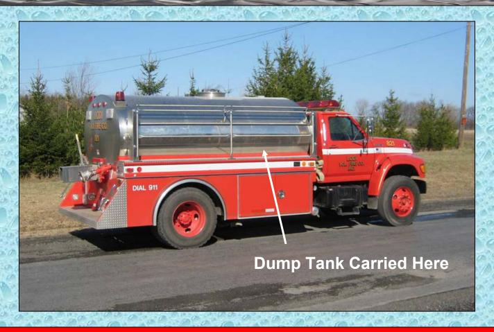
The tanker normally carries a 1,500-gallon dump tank. The photo above was taken at a water supply drill where the dump tank was being used.
