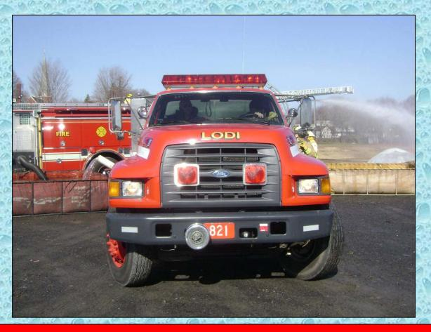
This smaller tanker can navigate the back-country roads pretty easily and with the 10-inch rear dump – it can offload its water very fast.
