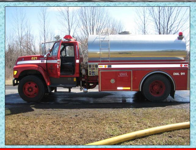
Tanker 821's 500 gpm pump is a PTO driven pump. The tanker also has a pre-connected attack line.
