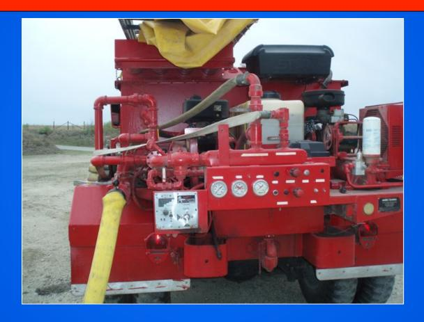
An Accufoam CAFS is the type of unit installed on Tanker 2.
