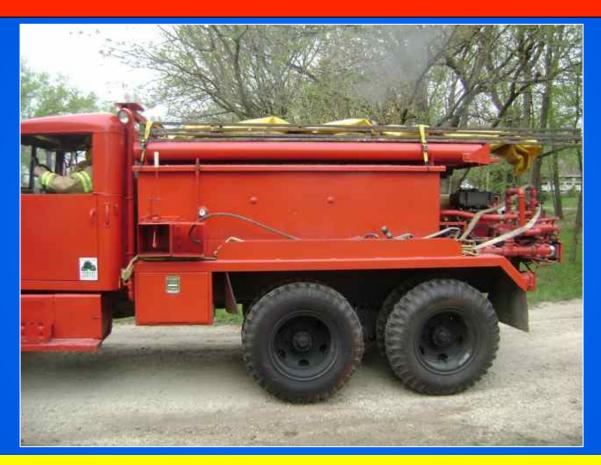
Besides carrying a 3,000-gallon dump tank (on top) – it is also equipped with several small forestry lines for supporting a fire crew.
