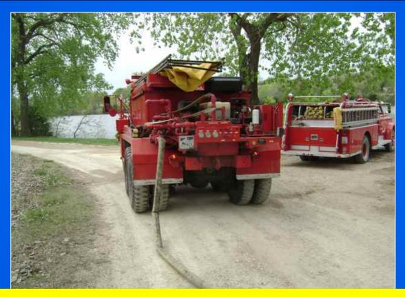
Tanker 2 is shown here getting filled at a water supply drill in nearby Marion. Looks like a bit more pressure is needed on that line – or better yet – some 4-inch hose. With a tanker that can dump its load in less in a minute – filling fast is key!
