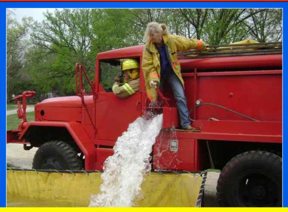
Tanker 2 has a single, 10-inch dump on the driver's side and when opened – dumps that 1,200 gallons in about 45 seconds!
