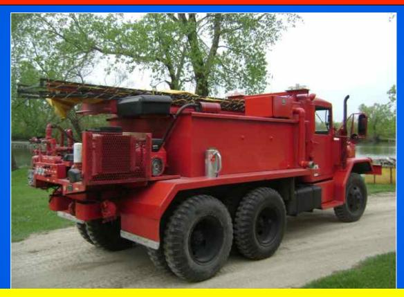
An interesting feature of this tanker is its CAFS capability. The unit has a small scale – but complete - CAFS component which provides this rig with a pretty darn good fire attack capability.
