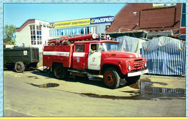
Looks like the pumper has seating for four or five and carries some fire fighting equipment in compartments and overhead.
