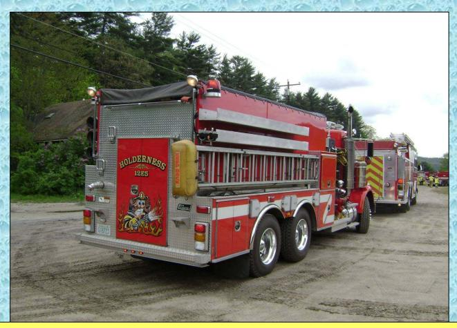
The engine/tanker carries a basic complement of engine company tools plus some additional suction hose.
