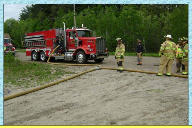
12-Engine-5 is shown above pumping a rural hitch set-up at a water supply drill in nearby Ashland, NH. The use of a double-clappered siamese is key to a successful rural hitch operation.
