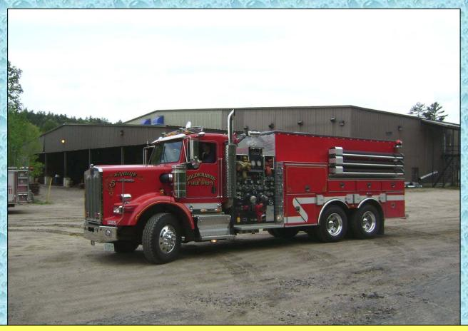
This 2006 engine/tanker is set-up to operate as either an attack engine or a water supply piece.
