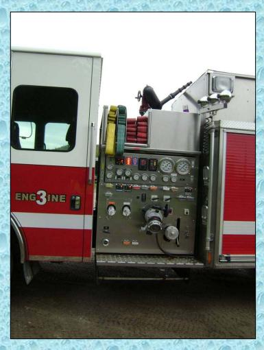
The 2,000 gpm pump on this rig allows it to flow big water as either an attack engine or a water supply piece.
