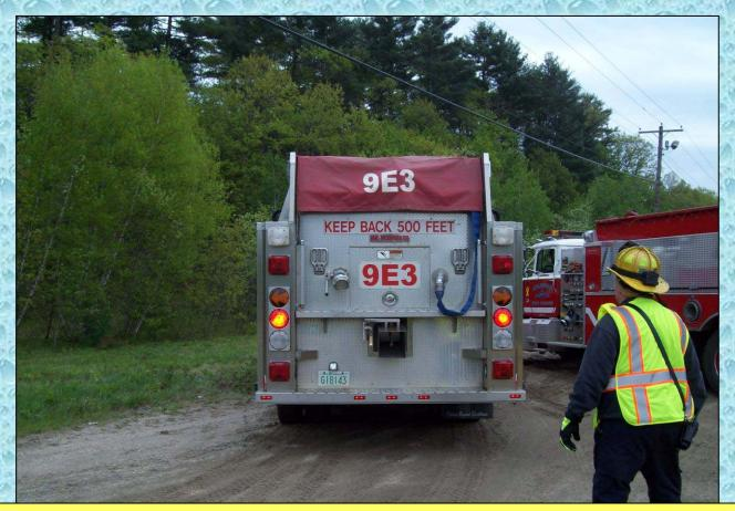
This 2005 engine/tanker is also equipped with a 10-inch rear dump and a 4-inch direct fill line.
