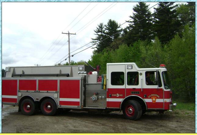
The engine/tanker is well-equipped for water supply and fire attack operations. In addition to the basic equipment it also carries Class A foam and a Turbo Draft.
