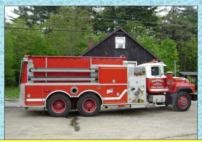
In terms of side dumps, the tanker has an 8-inch dump on each side making it quite versatile when hauling water.
