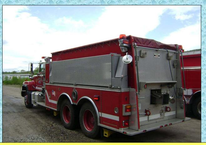
8-Tanker 1 carries two dump tanks – a 2,500 gallon and a 2,000 gallon.
