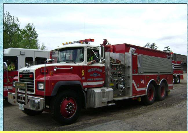
8-Tanker-1 carries 2,500-gallons of water and is equipped with a mid-ship mounted fire pump.
