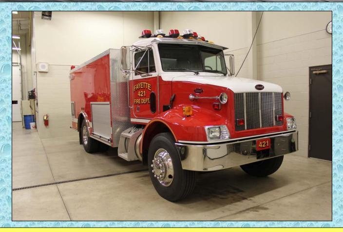
This 2004 "plastic" tanker is a compact, big water hauler! Its copolymer body allows for 2,400 gallons of water to be hauled on a single-axle.
