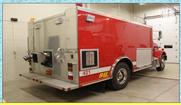
A unique feature of the design is that the tank is an integral part of the body. The rear and side dumps and large direct fill make this rig fast at loading and off-loading.
