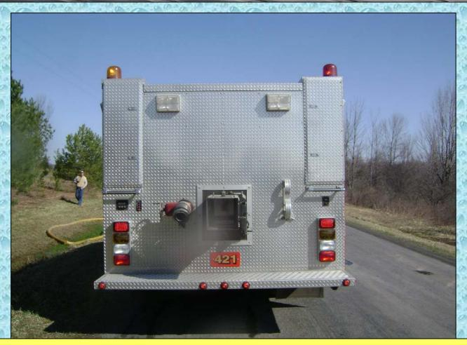
In addition to a 10-inch rear dump, Tanker 421 also has a 4-inch direct fill line and carries a portable dump tank (or "pond" as they say in the area).
