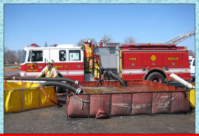
Crews are shown here using the pumper as the dump site engine at a recent water supply drill. The pumper is drafting and supplying Ovid FD's quint.
