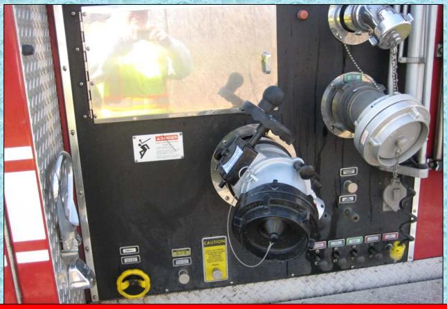
The pumper is outfitted with a TFT ball intake vale that is capable of high flow intake. The valve can also swivel to minimize kinking in the 5" LDH supply hose.
