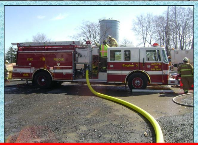
The pumper is shown above pumping a 5" supply line that is feeding a nearby quint that is flowing its 1,250 gpm pre-piped waterway.
