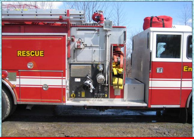
Engine 403 has a top-mounted pump panel and cross lays mounted in a tray configuration. The rig also has a high-flow discharge.
