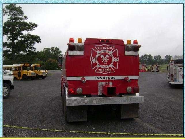
The rear of the tanker is where all of the water action takes place. The rig has a 10-inch Newton dump and two, 2-1/2-inch direct fill lines.
