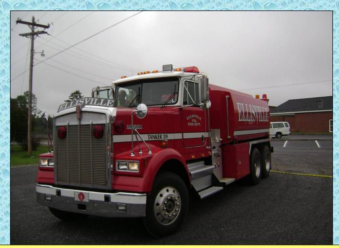
Tanker 39 is equipped with a 350 gpm pto driven pump which is capable of supporting a couple of handlines if needed.
