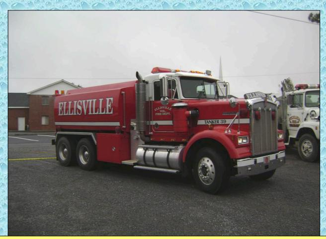
This 1987 tanker is a heavy-duty rig set-up to haul water. Its 3,000 gallons of water can make a big difference in a tanker shuttle operation.
