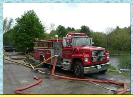
32-Engine-3 is shown above running a tanker fill site at a water supply drill in nearby Ashland, NH. The crew use additional suction hose and a portable pump to establish a 1,000 gpm flow for filling tankers.
