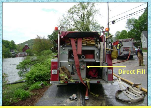
With 2,000 feet of 4-inch LDH, this pumper can support a long relay operation or a multiple supply line operation. The rig also has a direct fill line for its 1,000 gallon tank (seen in the middle just above the tailboard).
