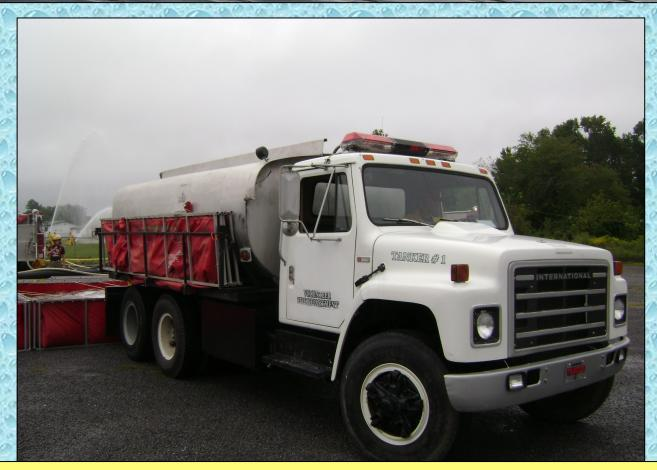
Tanker 1 carries a 2,500-gallon portable dump tank so that it can offload all of its water at one time and head to a fill site.
