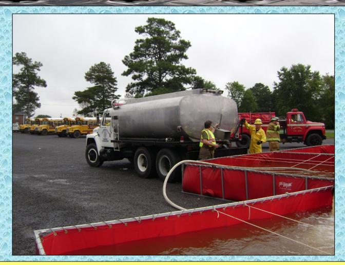
The tanker is shown here operating at a water supply drill in nearby Sylvania.
