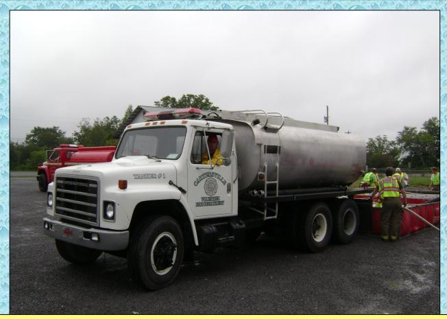
This 1980 tanker is built to work as a water hauling rig. It has no pump and carries little equipment – but it can certainly haul water!
