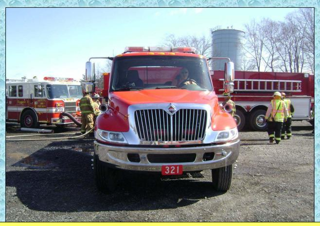
This 2,000-gallon tanker is built on a single-axle, International chassis.
