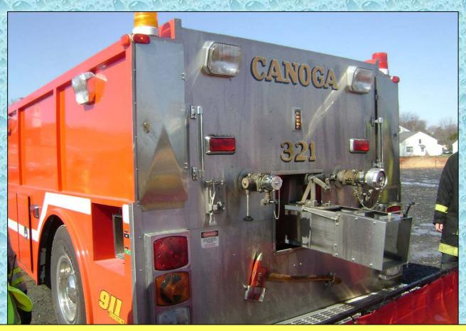
In addition to the rear dump, the rig also has two, 2-1/2-inch direct fill lines – one of which is outfitted with a 4-inch Storz adaptor – shown above.
