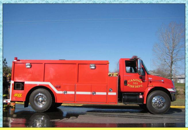
The tanker was fabricated locally and is designed to simply haul water. It carries a small, 250 gpm portable pump but uses its 10-inch dumps for offloading its water.
