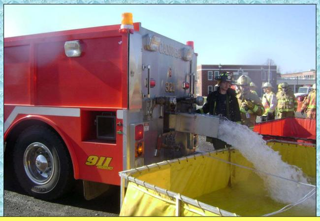
Tanker 321 is shown here dumping its water at a water supply drill in nearby Ovid, NY. This smaller tanker can offload very quickly and get back on the road for another load.
