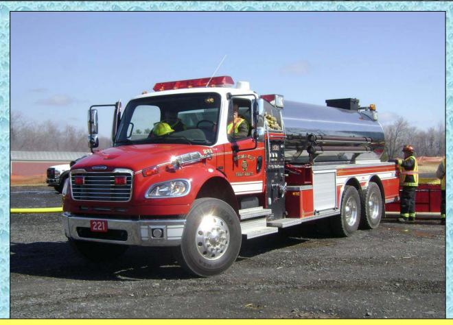
This 2006 tanker is built on a Freightliner chassis and carries 3,000 gallons of water and a 3,000-gallon portable dump tank.
