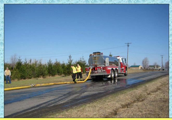
The tanker also has a 4-inch direct fill line and is shown above using that fill line during a water supply drill.
