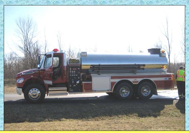
The tanker is a stainless steel wrapped poly tank that has both side and rear dumps – 10-inch in size.
