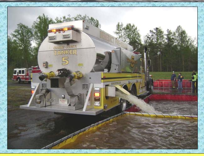
The automatic extensions on the dump chutes make side off-loading easy.
