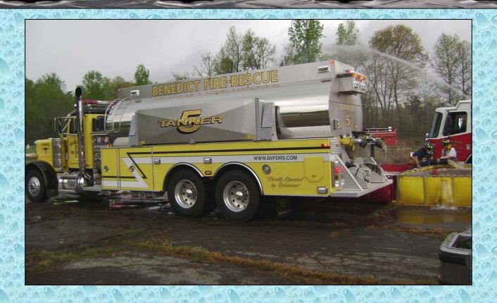
Built by 4-Guys, this elliptical poly-tank allows for a lower center of gravity and better road handling.
