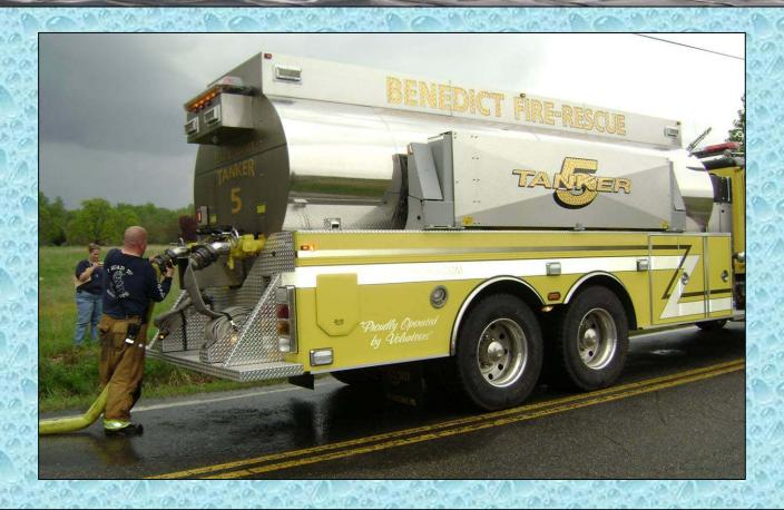
Tanker 5's dual, rear fills allow for reduced fill time. Here, a 5-inch line is connected to the direct fill.
