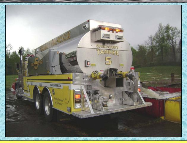
Tanker 5 is equipped with 10-inch side and rear dump chutes and carries two portable dump tanks.
