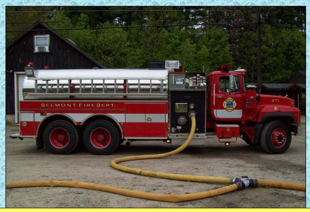
3-Tanker-1 is shown above pumping off its water into a rural hitch set-up at a 2009 water supply drill in nearby Ashland, NH. Three key items to consider when using the rural hitch are the size of the tank-to-pump line, the capacity of the pump, and the volume capability of the high-flow discharge.
