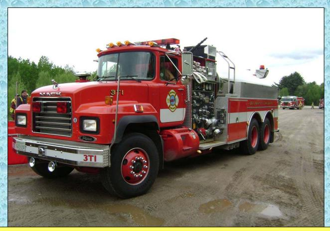
The rig carries a basic complement of engine company equipment but it is really more designed to function as a water hauling piece.
