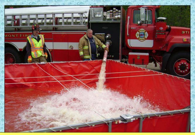
When no rural hitch is used, the unit must pump off its water using what some folks call a "ram horn." The one above is made of PVC pipe.
