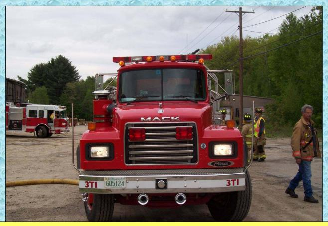
Belmont's 3-Tanker-1 is set-up to function in a "rural hitch" operation where tankers pump off their water instead of using portable dump tanks.
