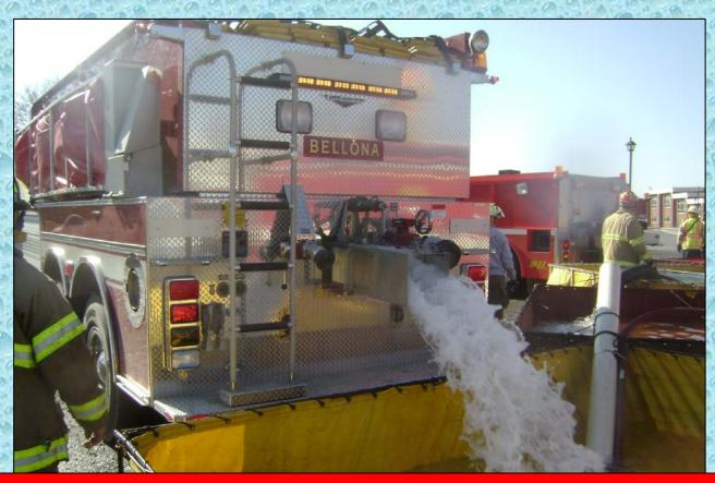
The tanker's 10-inch rear dump can offload the water in little time. The rig also carries 1,000-feet of 5-inch hose.
