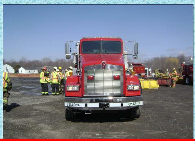
The Kenworth chassis and 500 hp Cummins motor provide plenty of load carrying capability.
