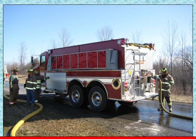
Shown here operating at a water supply drill in nearby Seneca County, Bellona's tanker gets filled through its large diameter direct fill line.
