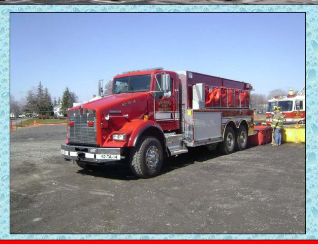
This 2008 tanker can haul some "big water" with its 3,000-gallon tank and dump valves on both sides and the rear.
