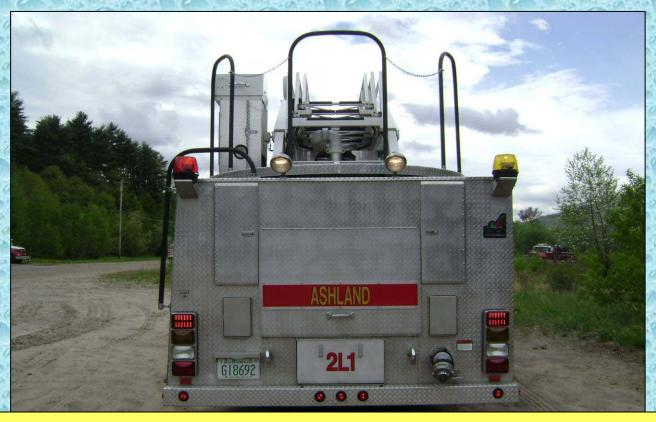
Of course, with most any hybrid vehicle there are trade-offs. With a quint, one trade-off is water tank size: the reason is the space needed for mounting the aerial device and its hydraulic system. In addition, ground ladder space can be limited for the same reason.
