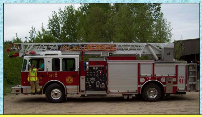
While the use of the "quint" concept is often debated in designing a municipal fire protection delivery system, quints do allow smaller departments to acquire aerial ladder capability combined with elevated master stream ability and additional pumping capacity. In some applications, this may help improve a FD's ISO rating.
