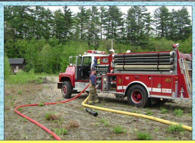
The pumper is equipped with a Hale, 1,500 gpm single-stage pump and carries more than the traditional 20-feet of hard suction hose.
