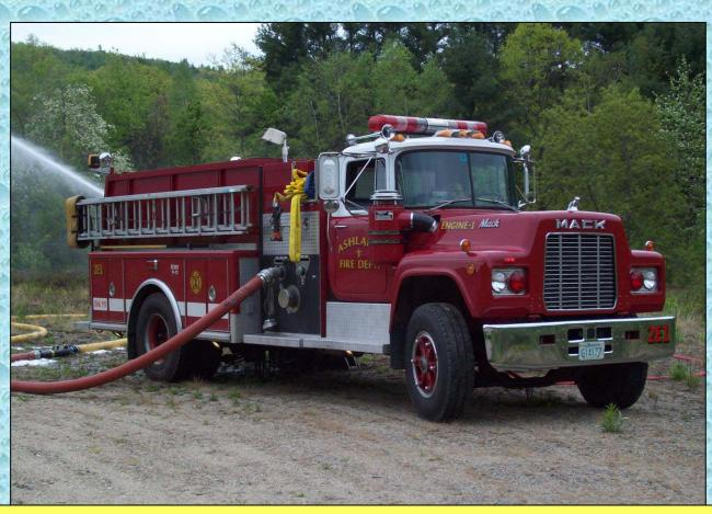
The pumper has a "high-flow" discharge so that it can pump to LDH without having to use special manifolds or other devices.
