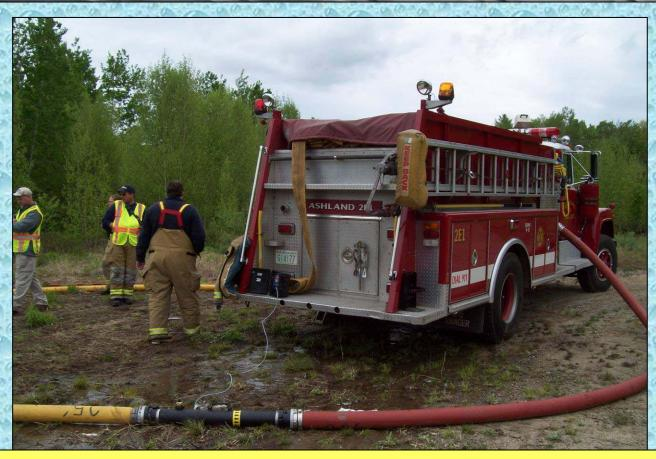
The rig carries 1,000 gallons of water and 1,000 feet of 4-inch supply hose; it also has several pre-connected attack lines. The pumper is shown hear working as the attack engine at a recent rural water supply drill.
