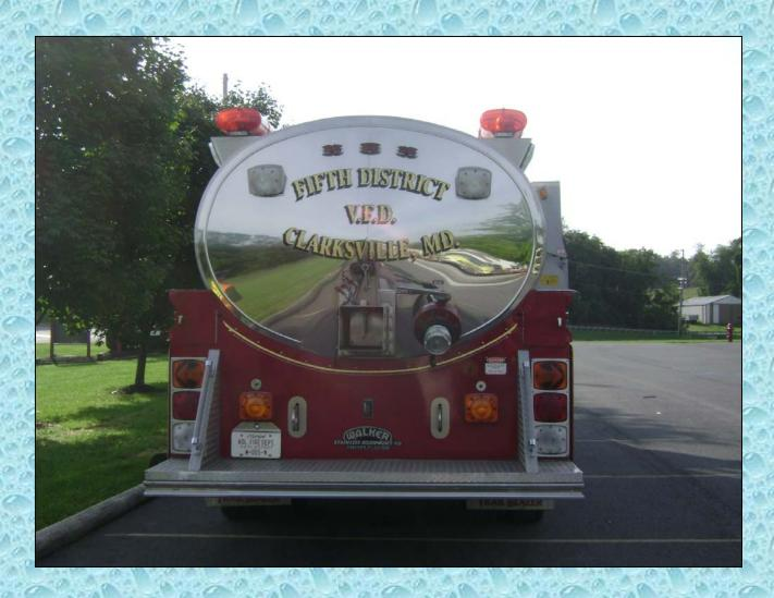
The rig was built by Walker Stainless and it is outfitted with a 10-inch rear dump and a 5-inch direct fill. These two features allow for quick dumping and quick filling – making this tanker a true water hauling beast.
