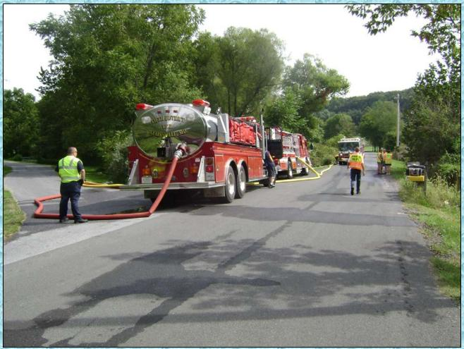
In the photo above, Tanker 5 is being filled through a single, 4-inch line at a tanker fill site.
