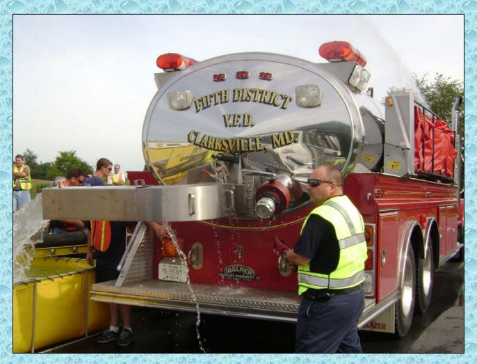
Shown here at a recent water supply drill in nearby Carroll County, Tanker 5 uses its detachable chute to perform a side dump operation.
