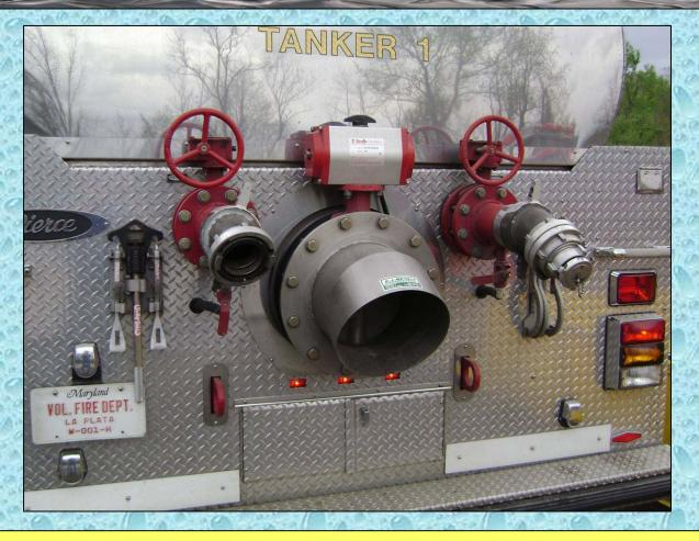
Perhaps the most impressive features of the tanker are the 12-inch dump and the dual, 5-inch direct fill lines.
