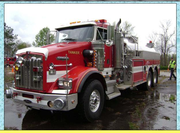
Tanker 1 is a really a 3,000-gallon elliptical tanker that has a 200-gallon foam "cell" in it. The rig is equipped with a Hale Qpak 750 gpm pump and has a couple of preconnect crosslays.
