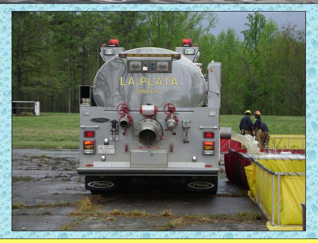
Shown here off-loading water via a side dump, Tanker 1 is set-up very nicely to off-load its water in a very short period of time.
