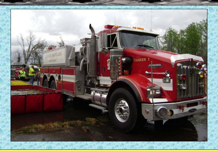
Tanker 1 is outfitted with large, side dumps and carries a 3,000-gallon dump tank.
