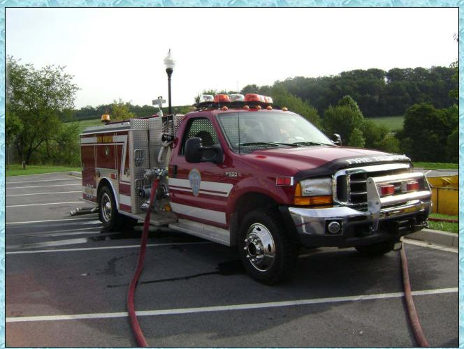
This 2000 KME mini-pumper is set up quite nicely to serve as a tanker fill-site unit. Its 1,000 gpm and 4-inch supply hose make it a versatile water supply support piece.
