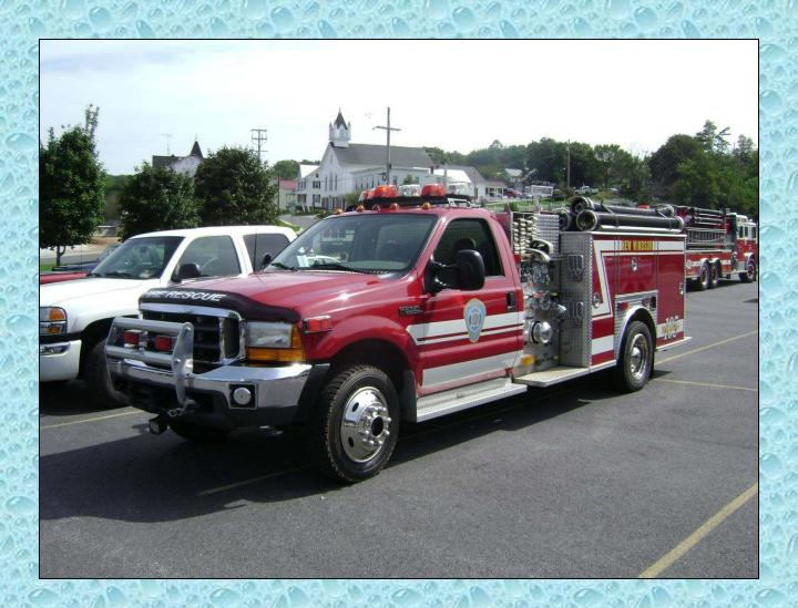
The rig was built by KME on a heavy-duty Ford 550 chassis and is powered by a diesel motor.
