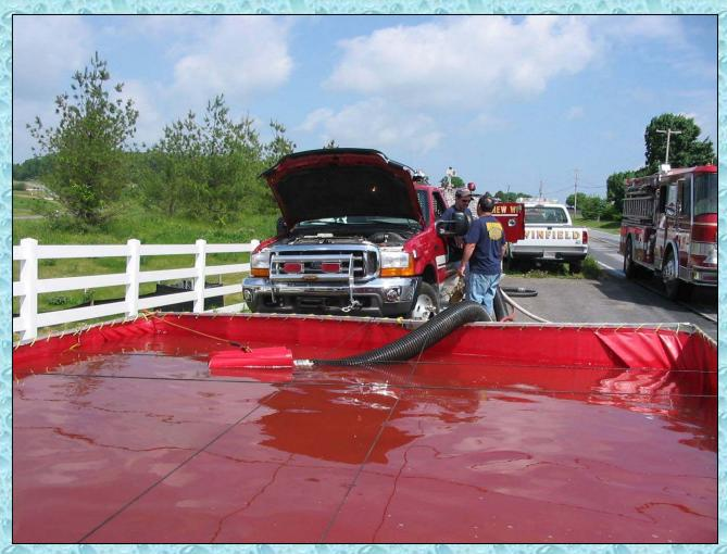
Brush 105 is shown above pumping jet siphons at a water supply drill in nearby Mt Airy. The unit has proven to very useful in operating jet siphons at dump sites – especially when the flow range approaches 1000 gpm and the primary drafting pumper can no longer support jet siphons.
