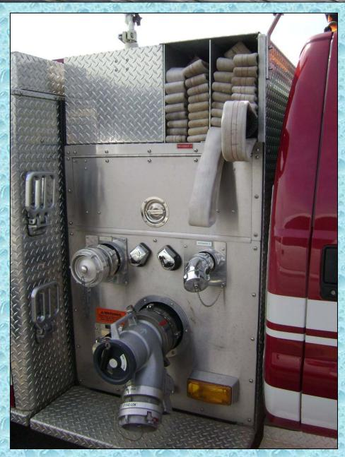
The unit is set-up to intake and discharge through 4-inch hose.
