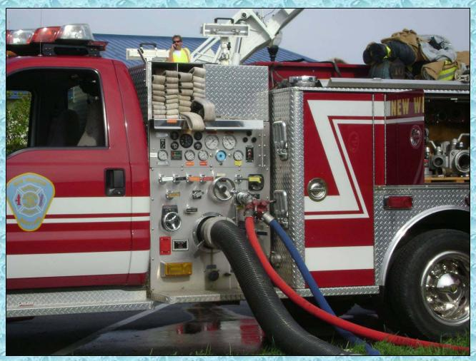
Brush 105 is equipped with a couple of pre-connected attack lines and some basic fire attack equipment.
