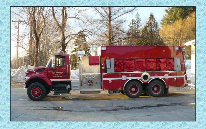
The tanker carries a 3,000-gallon dump tank and has a 10-inch round dump chute on each side.
