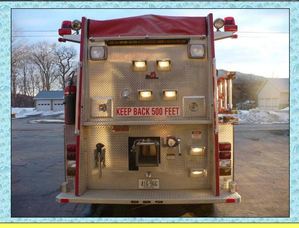
The tanker has a 10-inch rear dump with an extending chute. The rig is also equipped with a 2-1/2-inch direct fill line.
