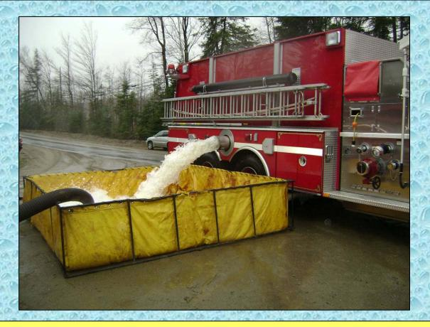
Engine 1 is shown above off-loading its water into a dump tank at a water supply drill in Strong. The big, side dump clearly illustrates the value of being able to offload fast from the side position.
