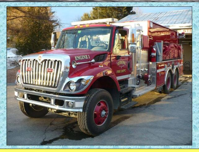
Engine 1 is a well-equipped engine/tanker that can function as an attack engine as well as a water hauling rig.
