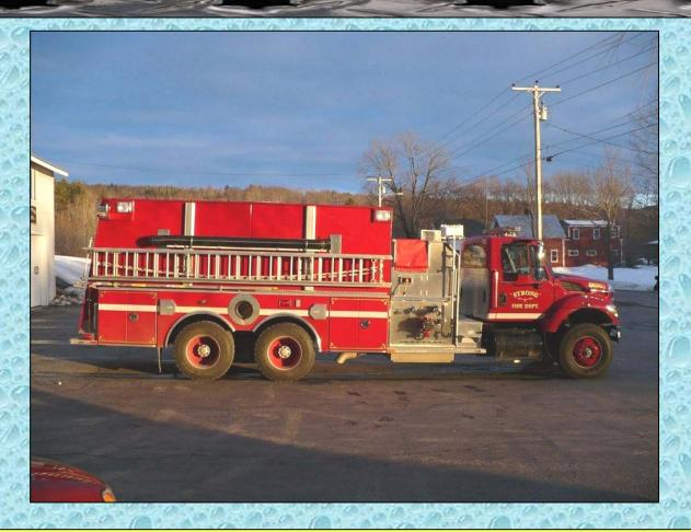
Engine 1 also carries a couple of pre-connected attack lines in the crosslay area so that the unit can function as an attack engine if needed.
