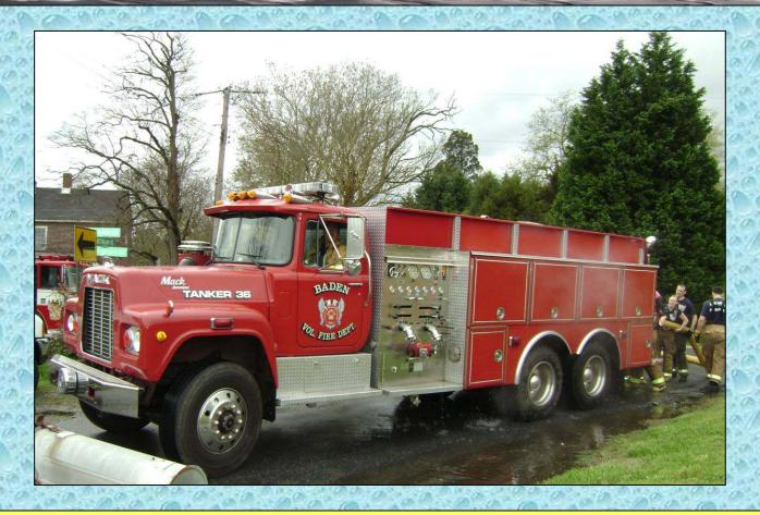
This 1986 tanker is built to work as a water hauling rig. It carries a minimum amount of fire fighting equipment – but it can certainly haul water!
