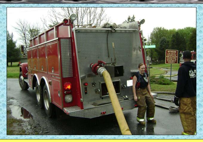
Tanker 36 (radio designation 836) is shown above being filled by a 5-inch line at a 2008 water supply drill in their community. This direct fill and the use of LDH make short work of the filling operation.
