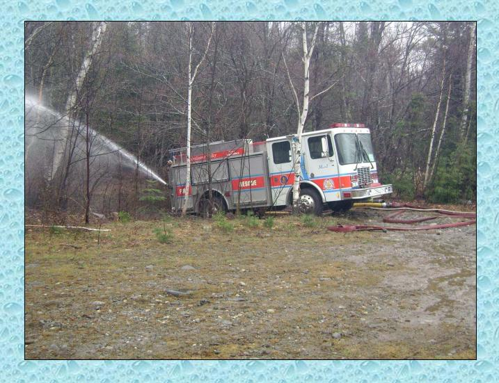
On big advantage of the rear-mount pump is accessing drafting sites. Shown here at a water supply drill in Strong, ME, Multi 1 backed up to a local stream and took suction to operate a tanker fill site.
