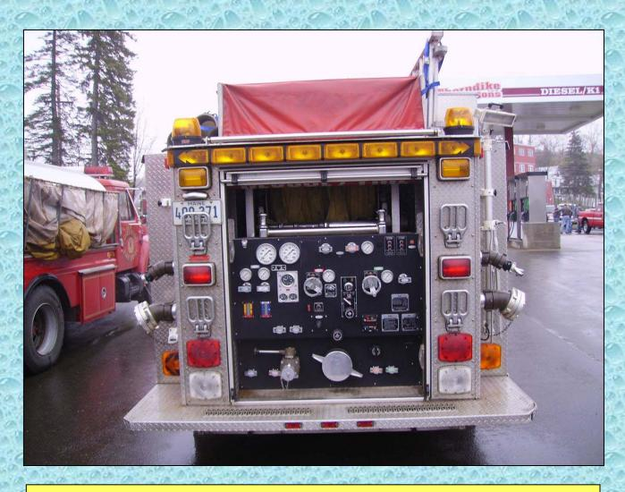
The unit is equipped with a 1,250 gpm, single-stage Hale pump with high-flow discharges. Note the reel of hose above the pump panel.
