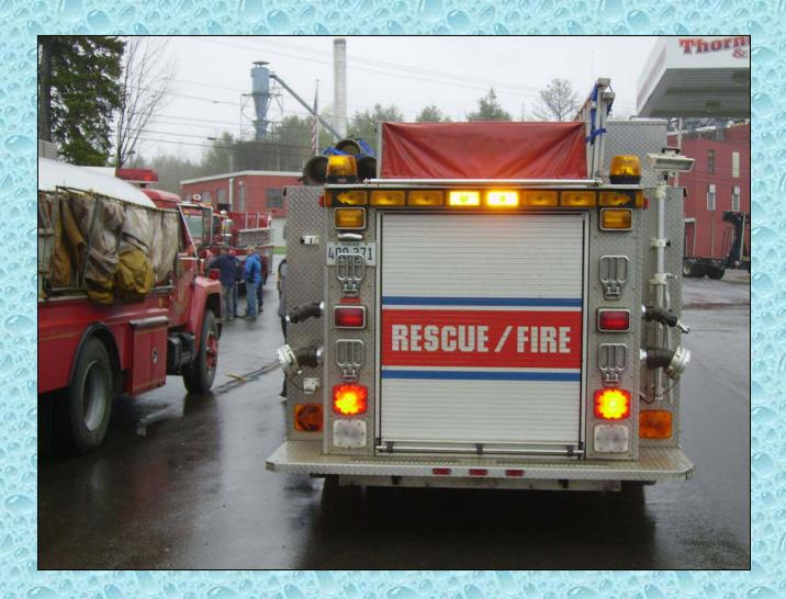
Multi 1 is very "European" in look with its rear, enclosed pump compartment and roll-up door. The unit also carries 4-inch LDH for supply line.
