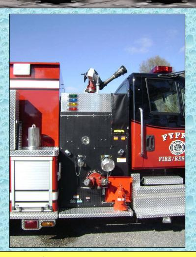
Engine 4 has a 1,250 gpm pump and is set-up to function as both an engine and a tanker if needed.
