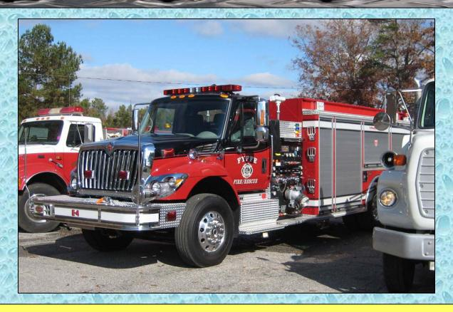
This 2008, KME engine/tanker was purchased to improve water supply operations for the Fyffe FD. The unit can function relatively well as either an engine or a water hauling rig and when combined with the department's 2,000-gpm engine – both units working together can deliver quite a punch.
