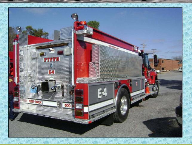
Engine 4 also carries a 2,500-gallon portable dump tank on the right side of the rig.
