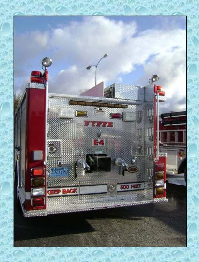
The engine/tanker is equipped with a 10-inch dump and dual, 2-1/2-inch direct fill lines. While none is shown in this photo, the rig can carry 1,500-feet of 5-inch LDH.
