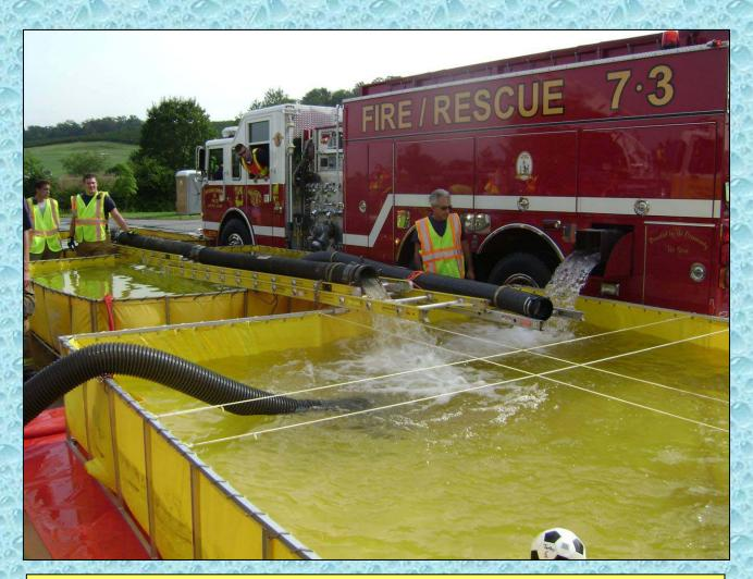
The engine tanker is shown here off-loading water at a water supply drill in Carroll County, Maryland. The large, side dumps allow for good positioning and reduce the need for backing.
