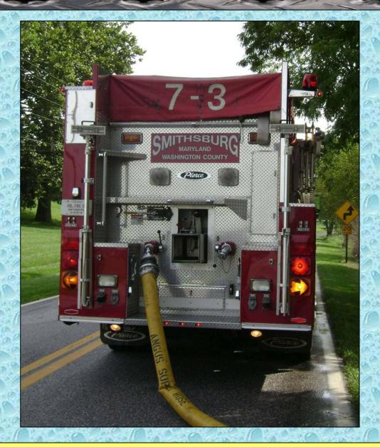
Here, the rig is shown being filled at a tanker fill site utilizing a 5-inch supply line. The use of LDH for tanker fill operations can significantly reduce fill times - thus allowing tankers to increase their delivery rates.
