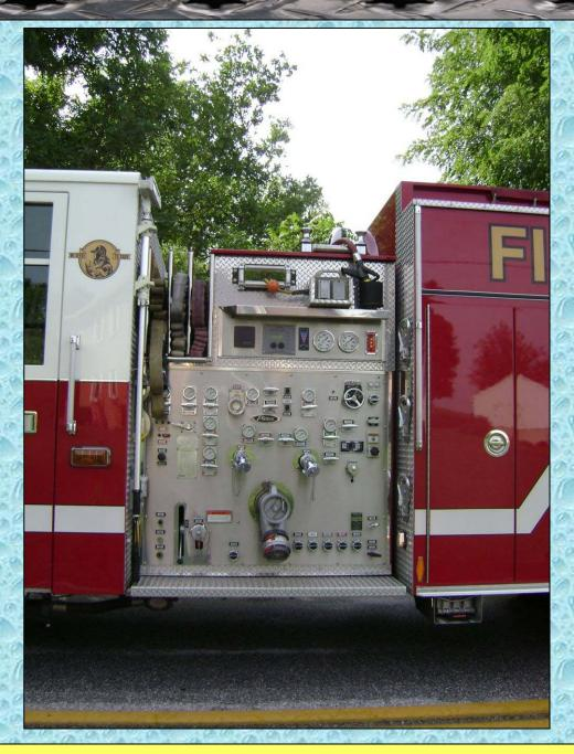
The rig is powered by a 500 hp Detroit diesel motor and has a Hale QFL, 1,250 gpm single-stage pump.
