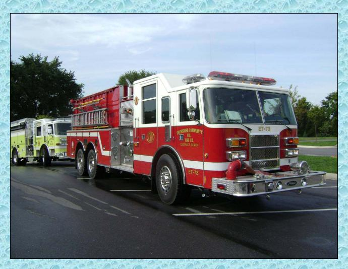
Engine Tanker 73 carries 1,400-feet of 4-inch hose and a 2,000-gallon dump tank.
