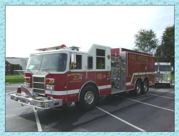
This 2000-gallon engine tanker is well-equipped to serve as either an attack engine or a water hauling rig. Built in 2000, Engine Tanker 73 serves the small community of Smithsburg, Maryland.
