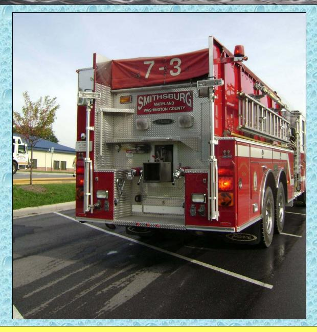
Engine Tanker 73 has a 10-inch dump on each side and one in the rear. The unit has dual, 2-1/2-inch direct fill lines which are also located on the rear of the vehicle.
