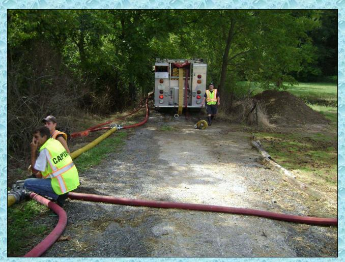
At the drill, the unit pumps to a 5-inch hose line which in turn is outfitted with a LDH manifold that is used to fill tankers as they arrive at the site.
