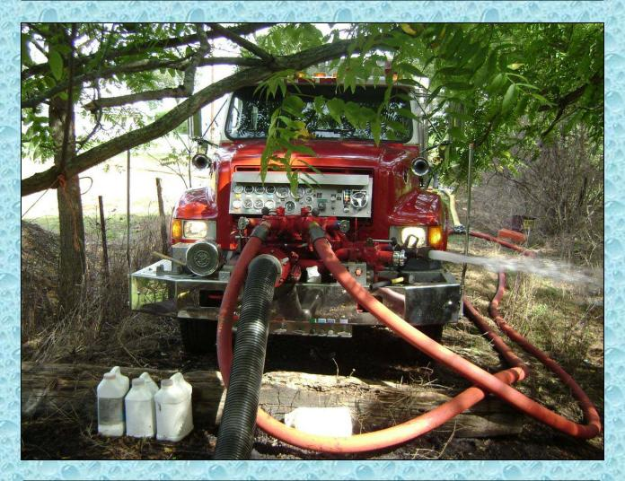
Engine 434's short wheelbase and 1,000 gpm front mounted pump make it a versatile piece for drafting. All of the photos in this presentation were taken at a 2008 water supply drill in nearby Carroll County, Maryland. Engine 434 was used to access a stream and establish a tanker fill station.
