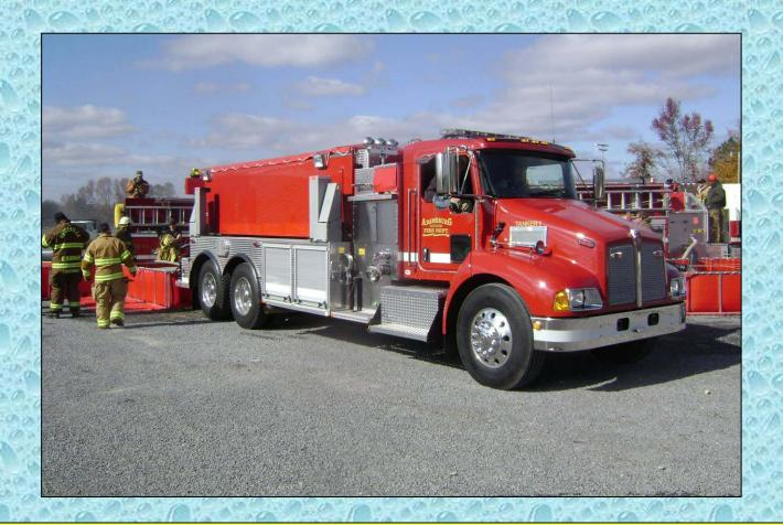
The tanker carries a 3,000-gallon dump tank and 1700-ft of 5-inch hose.
