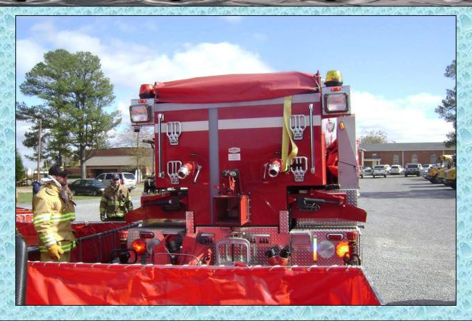
The tanker is equipped with a 10-inch rear dump plus a 10-inch dump on either side which makes the rig more versatile when it comes to off-loading water at a dump site.
