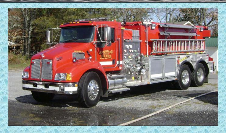
This 2007 tanker was one of a couple rigs purchased in DeKalb County, Alabama through the Federal grant process. While it basically serves as a tanker, the unit also carries a few, pre-connected attack lines and other firefighting equipment to allow it to function as an engine if needed.
