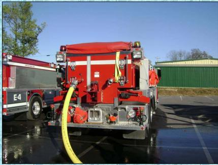
The tanker is equipped with two, 3-inch direct fill lines which allow the unit to be filled a couple of different ways. At a fill test conducted in Sylvania, AL, the single, 4-inch line proved to be the most efficient method for filling this tanker.
