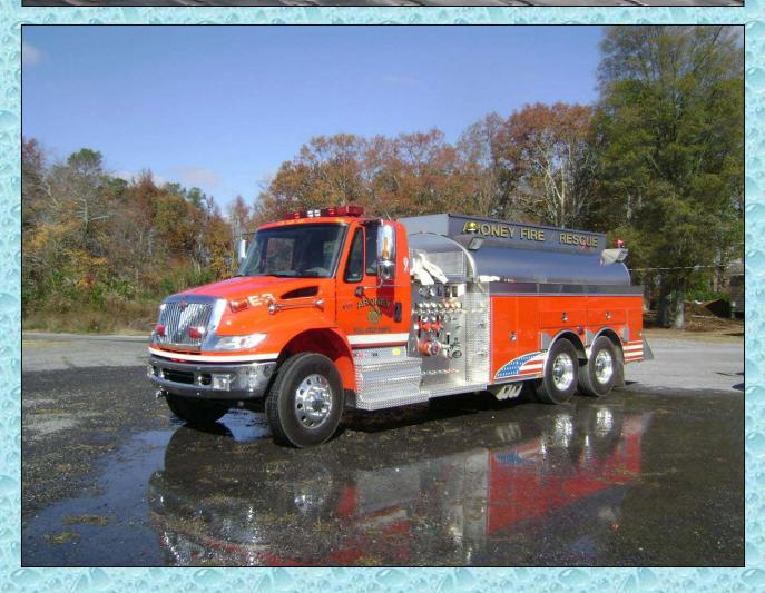
This 2007, elliptical tanker was one of a couple rigs purchased in DeKalb County, Alabama through the Federal grant process. While it basically serves as a tanker, it also carries a few, pre-connected attack lines to allow it to function as an engine if needed.
