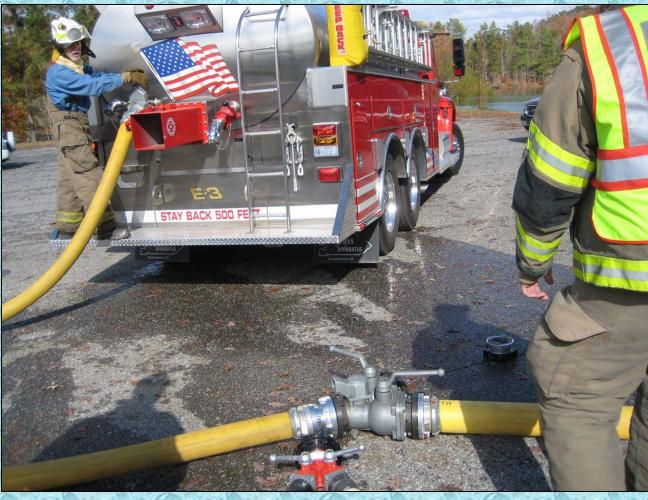
The rig is also equipped with both a 4-inch and a 2-1/2inch direct fill. The 4-inch direct fill is shown above being used at a recent rural water supply drill held in Sylvania, Alabama.
