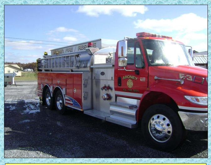
The vehicle is power by an International 330 hp diesel motor and has an automatic transmission.
