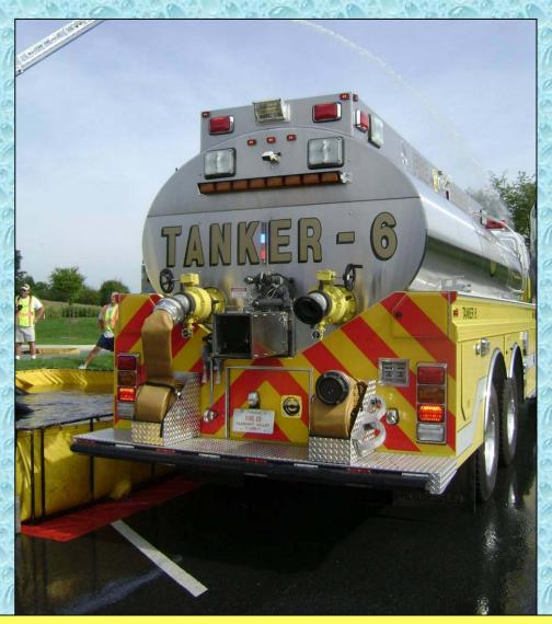
Tanker 6 has three, 10-inch square dumps that are controlled in the cab and on the exterior of the vehicle. The tanker also is outfitted with dual, 5-inch direct fill lines which allow for rapid filling.
