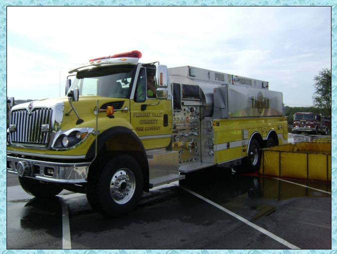
Tanker 6 is equipped with a 1,500 gpm pump so that it can serve as a nurse tanker if needed while a dump site is being set up.
