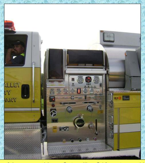
Tanker 6 is powered by a Caterpillar C13 motor and it is also outfitted with a few, pre-connected attack lines in case the tanker needs to serve as an attack piece in certain situations.
