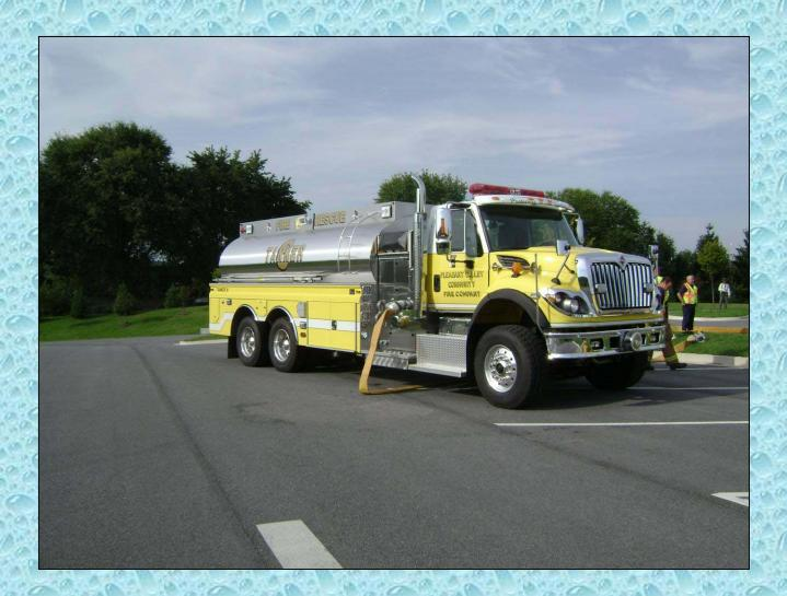
The rig's high-flow discharge allows it to directly support an attack engine if needed.
