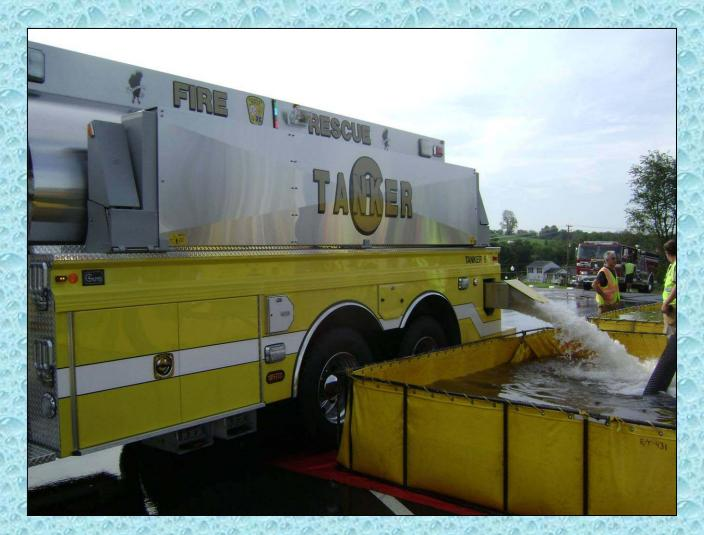
Shown here operating at a water supply drill in Carroll County, the 10-inch side dump allows Tanker 6 to offload very quickly.
