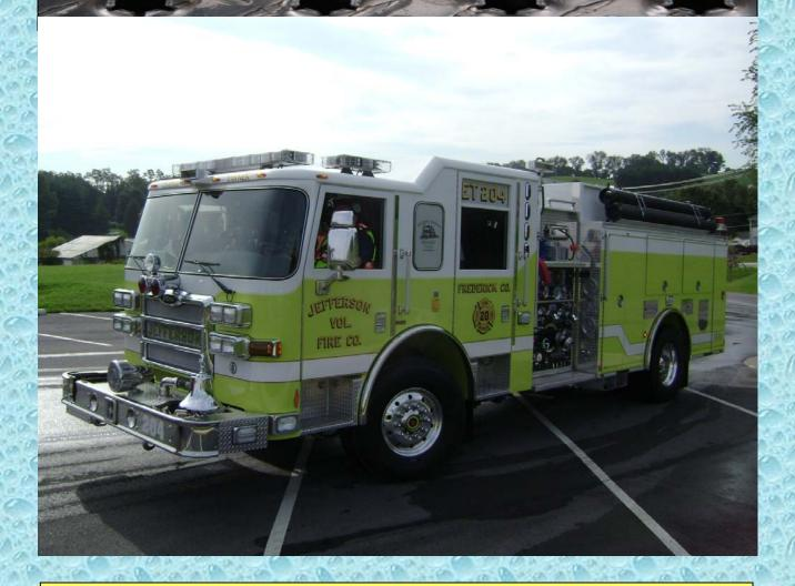
This 2008 unit serves primarily as an attack engine but also can operate as a tanker in a water shuttle operation.
