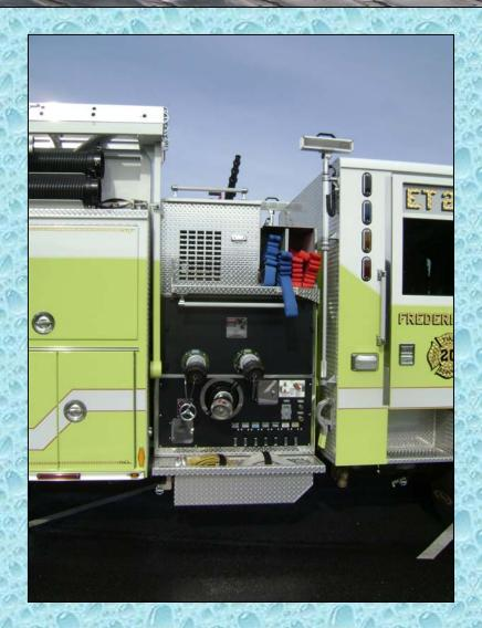
Dual, 4-inch discharges on the officer-side pump panel allow the rig to easily pump its maximum capacity.
