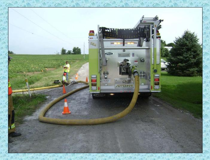
The engine tanker is shown here being filled at a tanker fill site. The rig is being filled through its 5-inch direct fill with 5-inch hose that is being supplied by an engine drafting from a farm pond 800-ft away.
