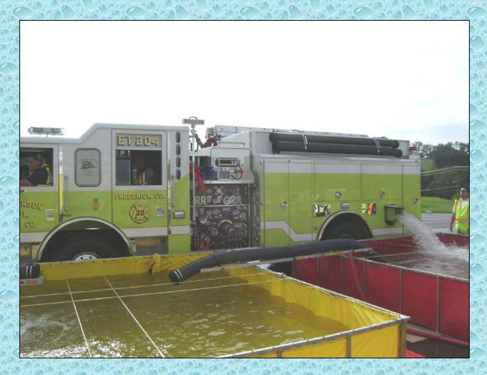
Engine Tanker 204 is shown here dumping water through one of its side dump chutes.
