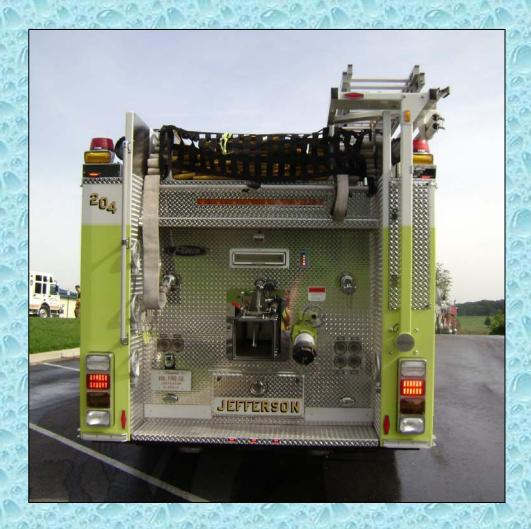
Engine Tanker 204 is equipped with a 10-inch Newton dump on the rear of the rig in addition to a 10-inch dump on each side. The unit also has a 5-inch direct fill.
