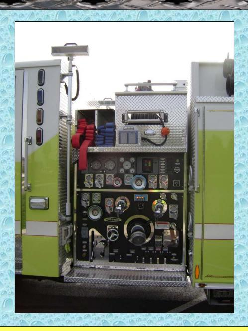
The engine tanker is outfitted with a Hale Q-Max 1,500 gpm pump equipped with MIVs and high-flow discharges.
