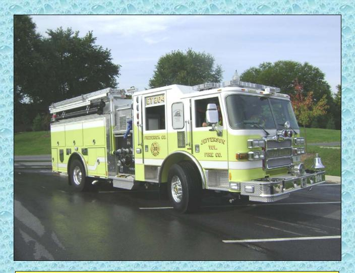
Engine Tanker 204 is powered by a Cummins motor rated at 525 hp. The unit carries 1,500-feet of 4-inch hose in addition to a full compliment of attack lines.
