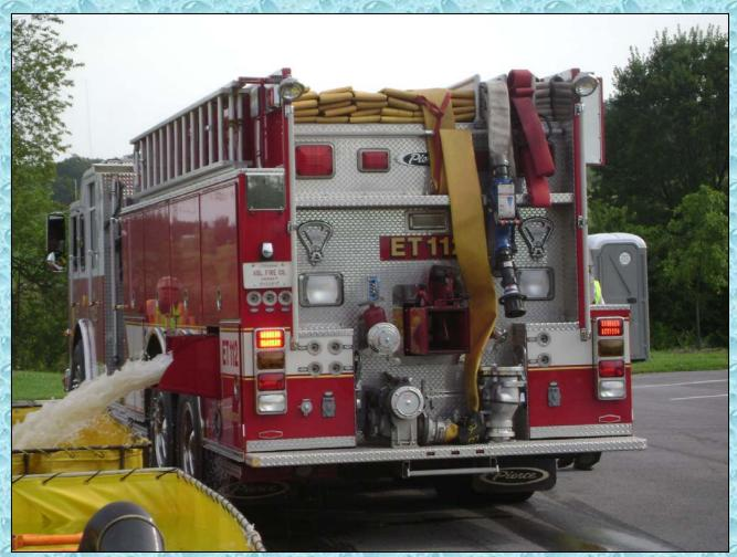
Engine Tanker 112 carries 1,200-ft of 5-inch LDH and is equipped with a pre-connected TFT Blitzfire line.
