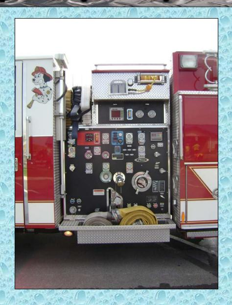
The rig was built by Pierce on a Dash chassis and is equipped with a 1,500-gpm Waterous pump.
