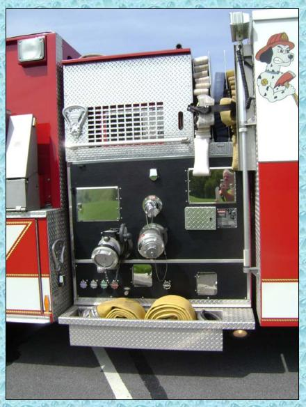
Engine Tanker 112 has a high-flow discharge on the officer side pump panel and is capable of flowing large volumes of water through 5-inch LDH.
