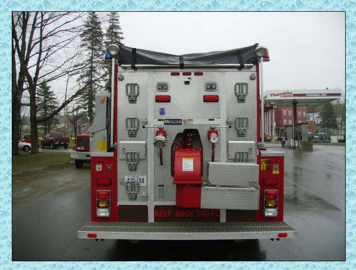
Engine 3 is equipped with a rather unique rear dump chute that pivots from side to side thus allowing flexibility in dumping.
