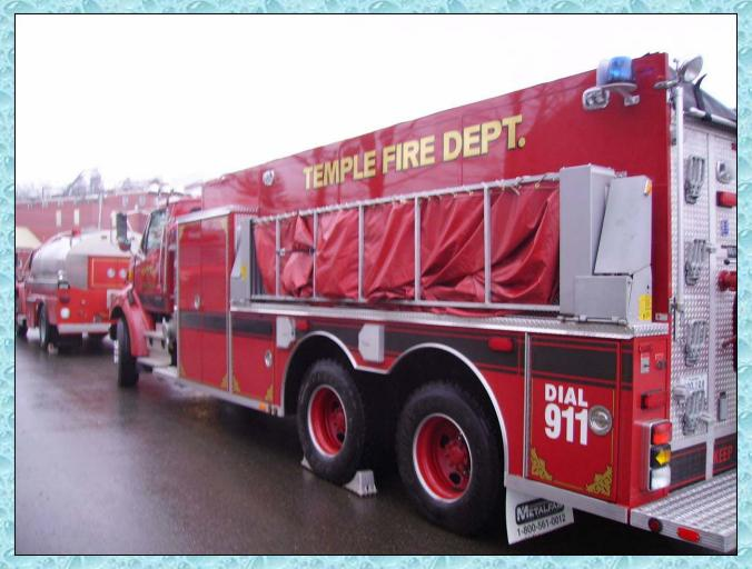
The 3,000-gallon dump tank is mounted on a hydraulic lift to make deployment easier.
