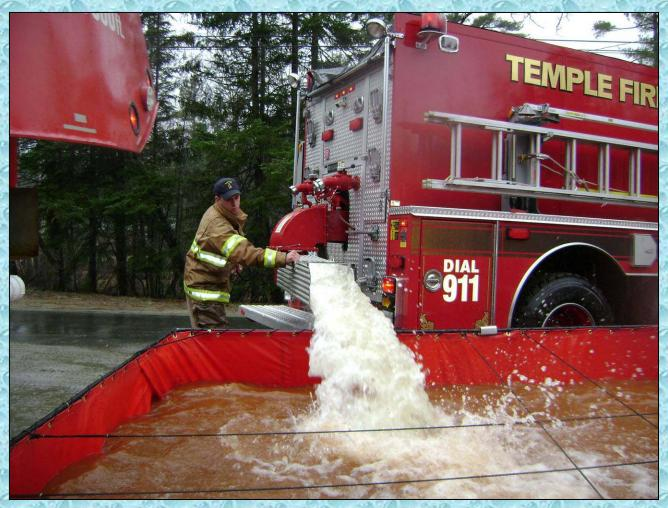
The 10-inch dump appears to work very well and with some guidance from a "worker bee", the water can be directed where needed even if the driver doesn't have "perfect" position.
