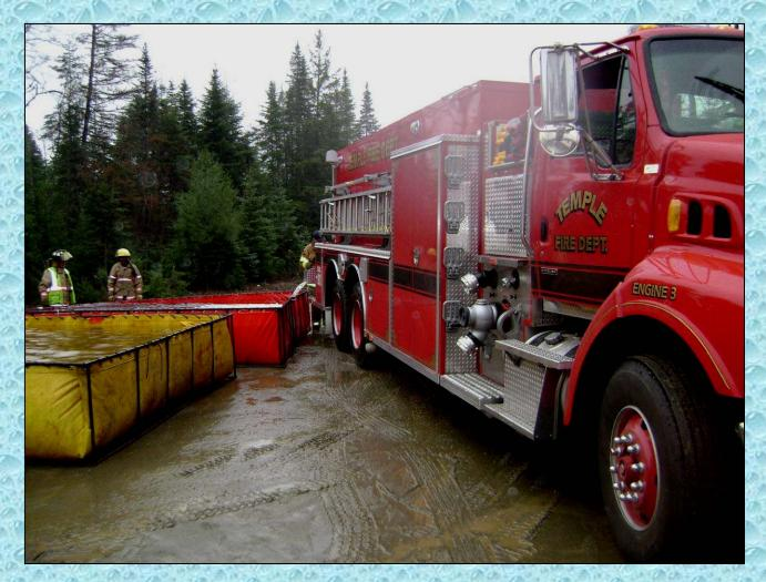
Shown here at a water supply drill in nearby Strong, Maine, Engine 3 offloads into one of the portable dump tanks.
