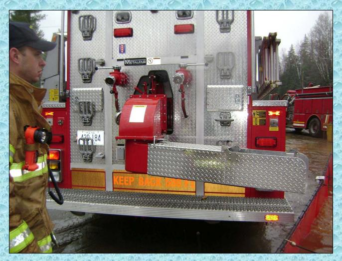
The pivoting, rear dump chute is shown deployed and ready for offloading.
