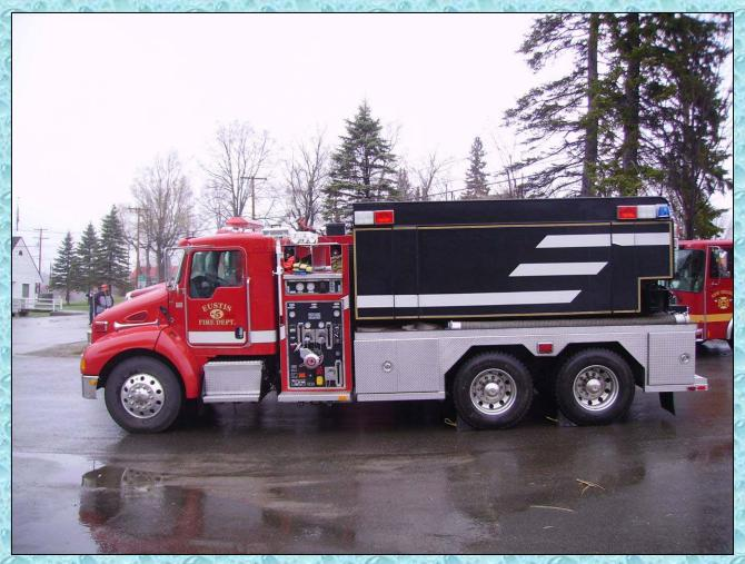
This 2007, T-shape tanker was one of a couple rigs purchased in Franklin County, Maine through the Federal grant process. While it basically serves as a tanker, it also carries a few, pre-connected attack lines to allow it to function as an engine if needed.
