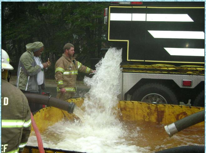
Shown here operating at a water supply drill in Strong, Maine, the 10-inch side dump allows Tanker 5 to offload very quickly.
