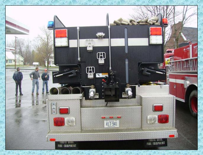
The tanker also is equipped with a rear, 10-inch dump valve and two, 2-1/2-inch direct fill lines. Although not all are shown in this photo, the tanker carries 40-feet of 6-inch suction hose and 900-feet of 5-inch supply hose.
