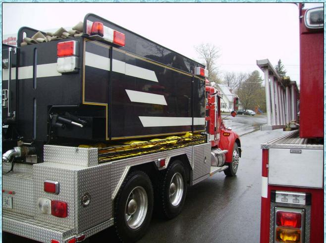
Tanker 5 is equipped with a 10-inch, square dump valve on each side of the rig and it carries a 3,000 gallon portable dump tank.
