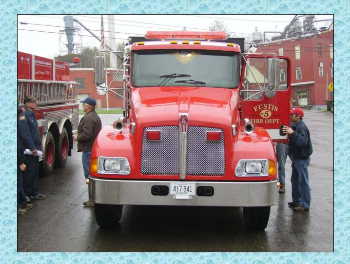
The rig was built by Ferrara Fire Apparatus on a Kenworth chassis and it is powered by an International diesel motor.
