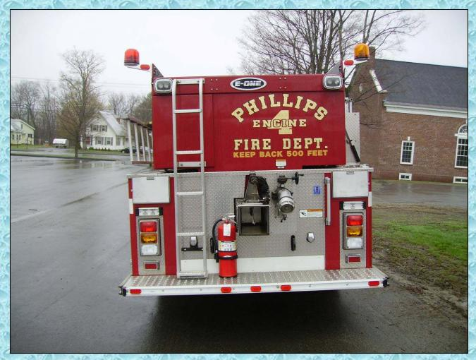
When shuttling water, Engine 4 can either dump through its 10-inch rear dump or through one of its 10-inch side dumps. The rig is also equipped with a 5-inch direct fill line.
