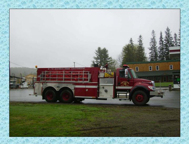
The rig is equipped with a 3,000-gallon dump tank and 20-feet of 6-inch suction hose. Engine 4 also has foam capabilities.
