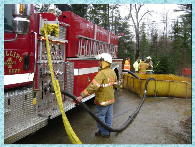
Engine 4 is shown here drafting through 2-1/2-inch suction hose to help increase its intake. Six-inch suction hose is already being used on the officer's side to take suction from another portable dump tank.
