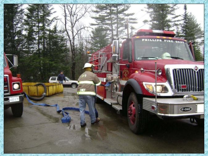
Shown here at a drill in Strong, Maine, Engine 4 sets up at the dump site and begins to supply water to the attack engine while the dump tanks are being put into position.
