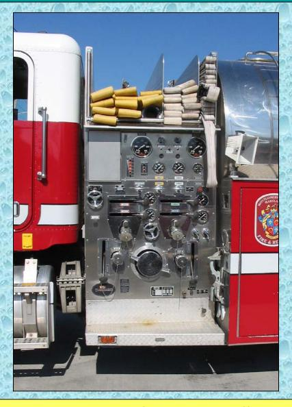
The 1250 gpm pump allows for pumping off the tanker's water until a dump tank operation can be established.
