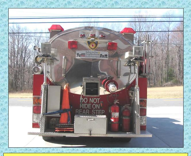
Tanker 714 is outfitted with a 10-inch Ziamatic, square dump on the rear of the rig.
