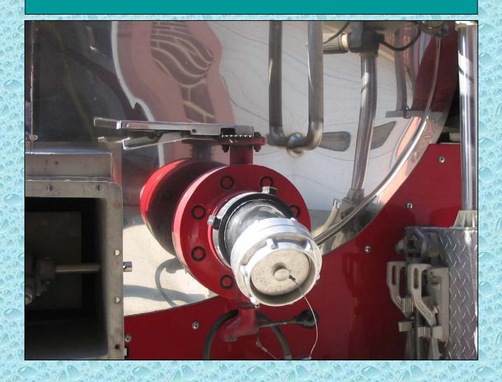
Nothing fancy here. A plain old butterfly valve controls this intake. Simple and reliable.
