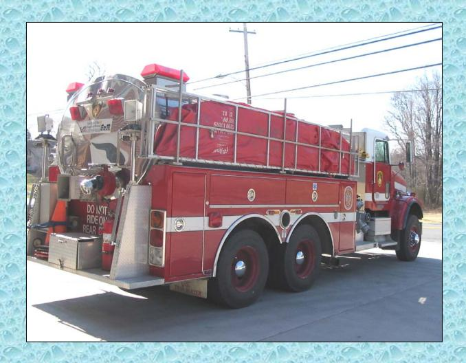
Tanker 714 carries a 4000-gallon dump tank which is large enough to hold the tanker's contents. This is important in a tanker shuttle operation – we don't want to wait to dump all of the water. We want to dump and move!
