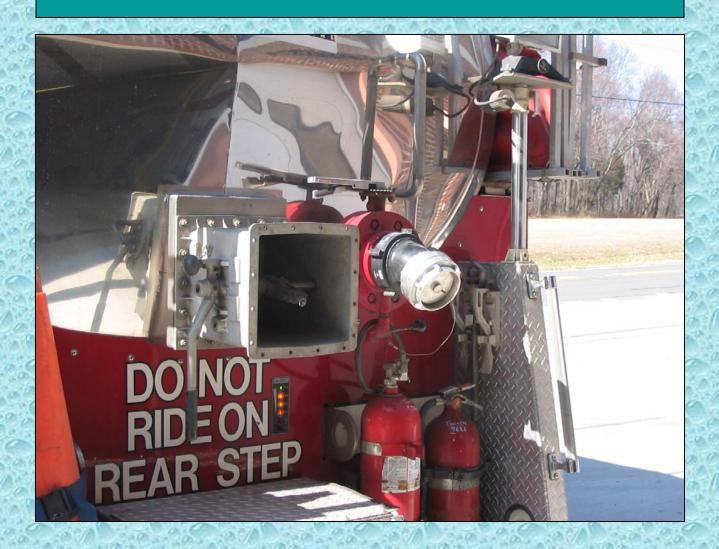
The tanker is also equipped with a 5-inch direct fill-line.
