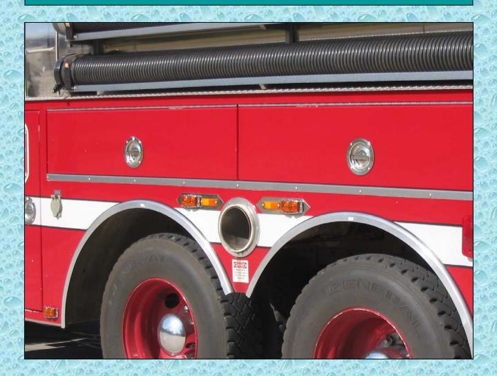
Tanker 714 is equipped with 8-inch, round side dumps that have extending tubes. They are controlled remotely.
