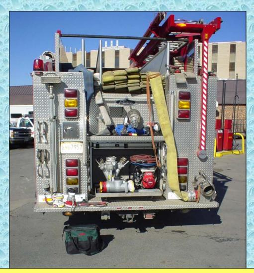
The rear-end of RE703 is set-up to handle water supply business. Besides the bed of LDH, there is also several LDH appliances and a pre-connected TFT Blitzfire nozzle.
