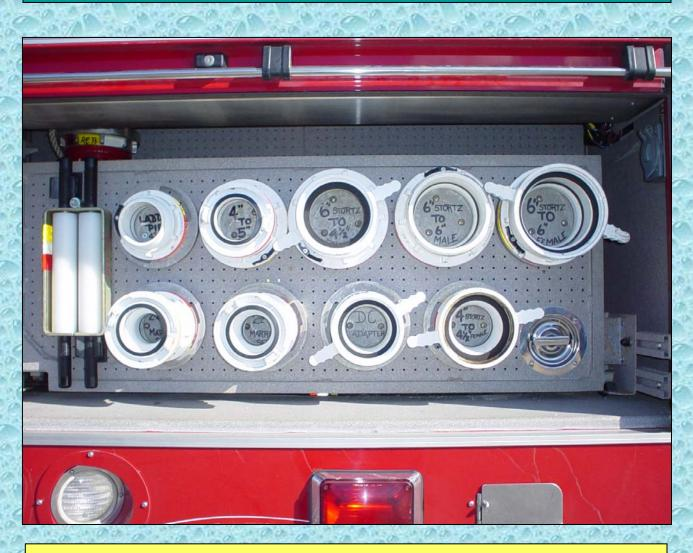
Adaptors are critical in any large scale water supply operation. On RE703, adaptors are clearly labeled and readily accessible.
