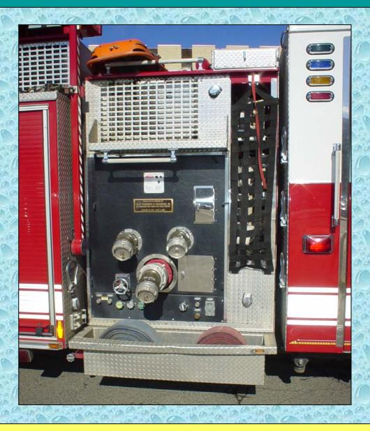
Dual, 4-inch discharges on the officer side allow for large capacity pumping operations.
