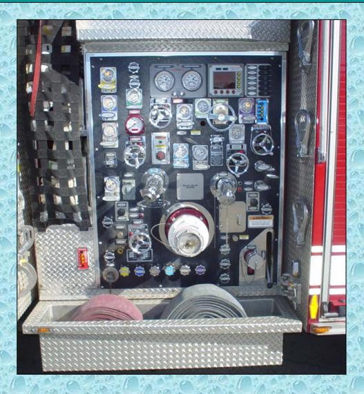
The pump panel is well laid out and the 6-inch suction intake is outfitted with a Hale MIV. Note the Storz fitting already in place.
