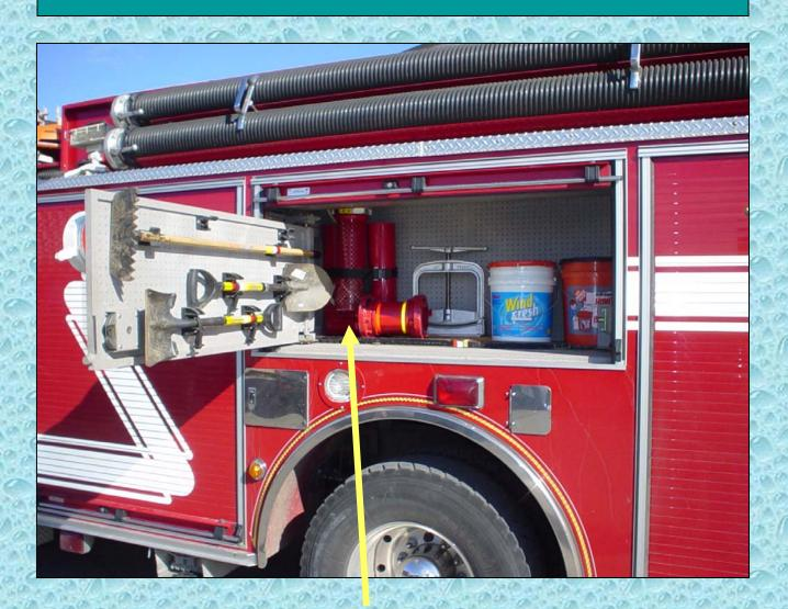
A swing out divider provides access to the floating strainer and jet siphon.
