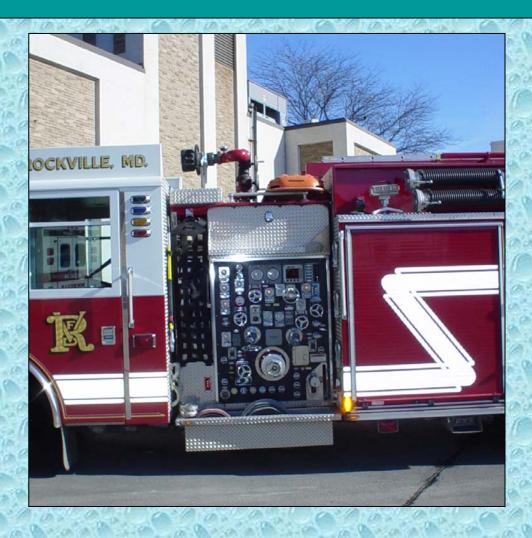
The rig is outfitted with a Hale QMax 2000 gpm single stage pump. It also has a pre-piped deck gun that is trimmed out with a TFT nozzle capable of flowing 2000 gpm.
