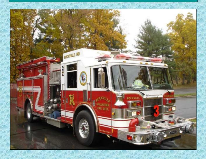
This 2000 gpm pumper was designed to support both vehicle extrication operations and water supply operations.
