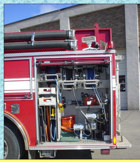
For extrication operations, the rig is equipped with Amkus hydraulic rescue tools.
