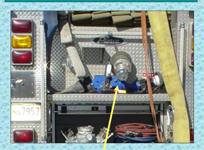
One unique feature of RE703 is the 5-inch rear intake that can serve as either an intake or a discharge based upon the positioning of a control valve by the pump operator.
