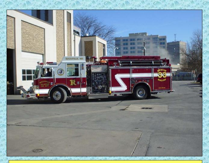
Rescue Engine 703 is a 2003 Pierce pumper built on a Dash chassis.
