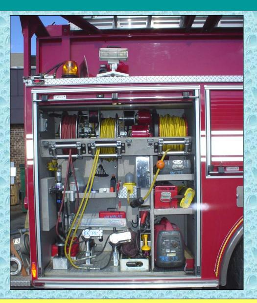
The officer's side of the rig is also equipped with extrication equipment.
