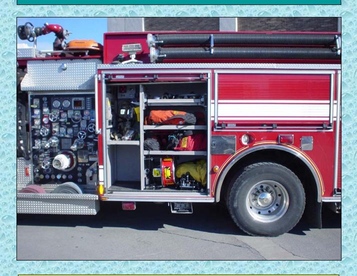
The rig is equipped with a myriad of tools and appliances to handle numerous types of water supply and vehicle rescue scenarios.
