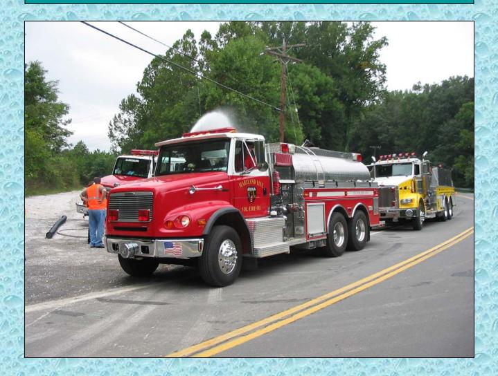
This elliptical tanker is designed to run on the rolling hills of Baltimore County, MD. The tank design allows for a lower profile which improves the handling of the vehicle over the local terrain.
