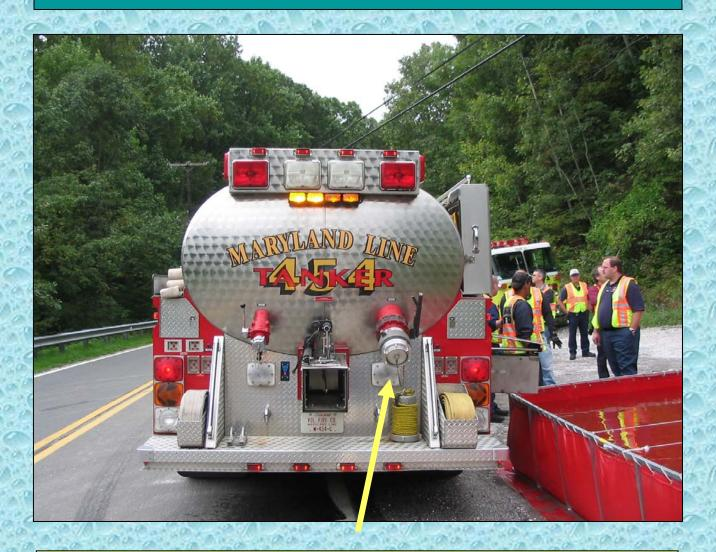
Shown here in action at a local water supply drill, Tanker 454 is equipped with both a rear and side dumps as well as a large, capacity direct fill line on the rear.
