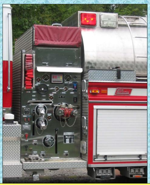
The rig is also equipped with a 1000 gpm single stage Darley pump.
